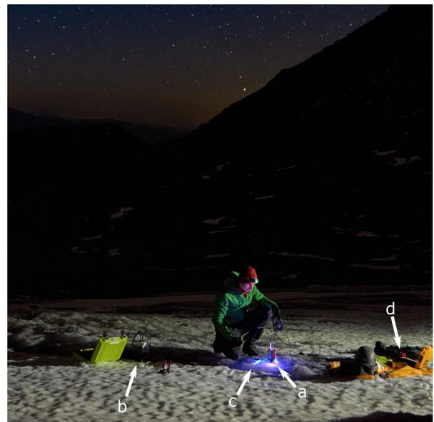
Fig. 2. Backscattered blue light can be seen right below the laser (a). The PMT is positioned to the left (b). A GPS receiver is co-located with the laser (c). The DAQ remains in its hard case (d).
