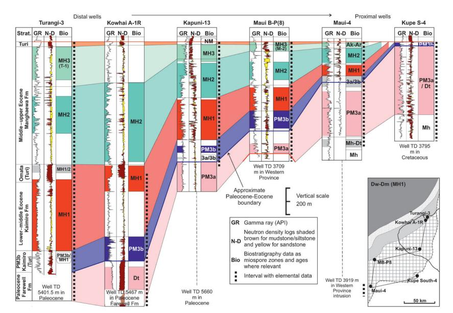
Fig. 3. (Colour online) Cross-section showing chronostratigraphic framework for the study wells; location of the transect is shown on the inset map, with legends on Figures 1 and 2 for facies belts and biostratigraphic data, respectively. Intervals sampled for geochemical analyses are indicated; mudstone/siltstone intervals are indicated by brown shading on the neutron-density (N-D) log crossover.
