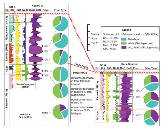
Fig. 10. (Colour online) Relative proportions of feldspars from QEMSCAN data (Higgs *et al.* 2012*b*) with bulk-rock elemental data (this study) plotted against gamma-ray (GR) and biostratigraphy (Bio) data for wells Kapuni-13 and Kupe South-4. Fdsp refers to total feldspar abundance (vol%) to nearest percent; relative proportion of feldspar types are illustrated by pie charts.
