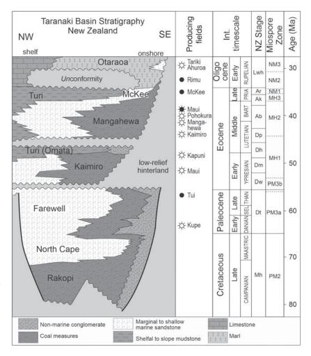
Fig. 2. Cretaceous and Palaeogene stratigraphic framework for the Taranaki Basin, New Zealand, plotted against the geological timescale and correlative miospore zones. The stratigraphic framework is modified from King & Thrasher (1996), international timescale from Gradstein et al. (2012) and miospore zones from Raine (1984, 2004). Dt - Teurian; Dw - Waipawan; Dm -Mangaorapan; Dh - Heretaungan; Dp - Porangan; Ab - Bortonian; Ak - Kaiatan; Ar - Runangan; Lwh - Whaingaroan.
