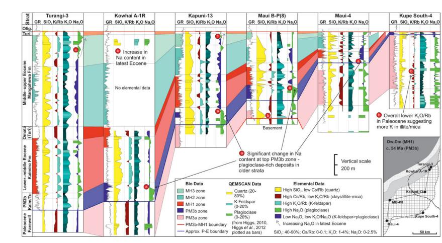
Fig. 8. (Colour online) Cross-section through study wells showing vertical changes in SiO<sub>2</sub>, K<sub>2</sub>O/Rb, K<sub>2</sub>O and Na<sub>2</sub>O plotted against gamma-ray (GR), biostratigraphy (Bio) and QEMSCAN data. Mudstone/siltstone cuttings are indicated by brown shading on K<sub>2</sub>O/Rb data.
