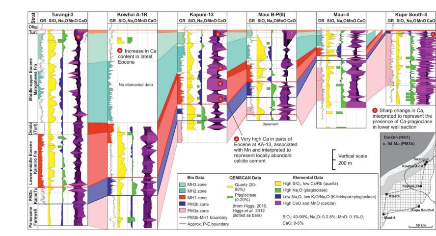
Fig. 9. (Colour online) Cross-section through study wells showing vertical changes in SiO<sub>2</sub>, Na<sub>2</sub>O, MnO and CaO plotted against gamma-ray (GR), biostratigraphy (Bio) and QEMSCAN data.
