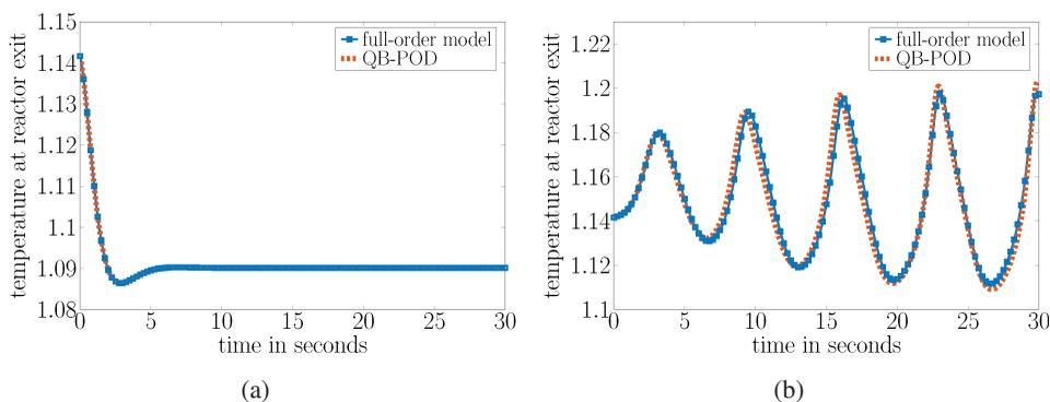
Figure 9.1. Model reduction results for tubular reactor of Kramer and Willcox (2019, Figure 5). The reduced model uses lifting to quadratic-bilinear (QB) DAE form,  $r_1 = 30$  POD modes to approximate the differential equations and  $r_2 = 9$  POD modes to approximate the algebraic equations. (a)  $\mathcal{D} = 0.162$  (stable case). (b)  $\mathcal{D} = 0.167$  (unstable case).
