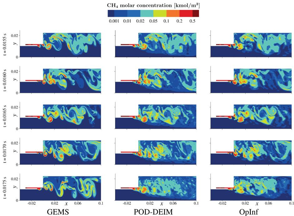
Figure 9.4. Model reduction results for the single-injector rocket combustion process of *McQuarrie et al. (2021, Figure 8)*. Molar concentrations of  $\text{CH}_4$  produced by GEMS (308 184 dof, left column), POD-DEIM (70 dof, middle column), and OpInf (43 dof, right column). POD basis computation and reduced model training used the first two milliseconds of data. (Figure reproduced with permission. Copyright © 2021 Taylor & Francis Ltd., [www.tandfonline.com](http://www.tandfonline.com).)
