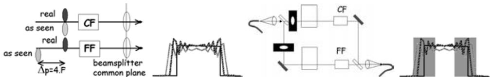
**Figure 2.** from left : axial separation ( $F$  : focal length in CF) for images of input pupilla on each interferometer arm as seen from recombining plate, illustration of resulting wavefront mismatch, insertion of “corrective” stops, “cleaning” effect of stops.
