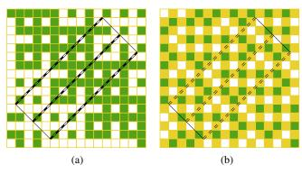
FIGURE 20. (Colour online) (a) Two  $G_1$  lattice units = one  $H_1$  lattice unit of an order-40 isonemal prefabric of species 6 that falls apart. (b) Partial construction of a fabric that could be coloured to look like the design of (a). Dark and pale cells as required before striping, formerly redundant cells neutral.
