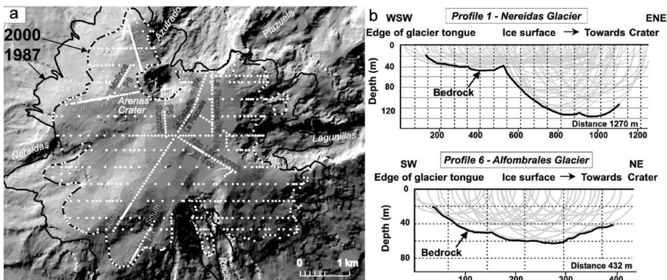
**Fig. 7.** Topographic DEM of the Ruiz summit. (a) Boundaries of the ice cap in 1987 and 2000, lines along which ice thicknesses were measured with a portable impulse radar, and GPS interpolated points for cross sections. (b) Two ice thickness profiles show ellipses measured from electromagnetic waves across the Nereidas and Alfombrales glaciers.
