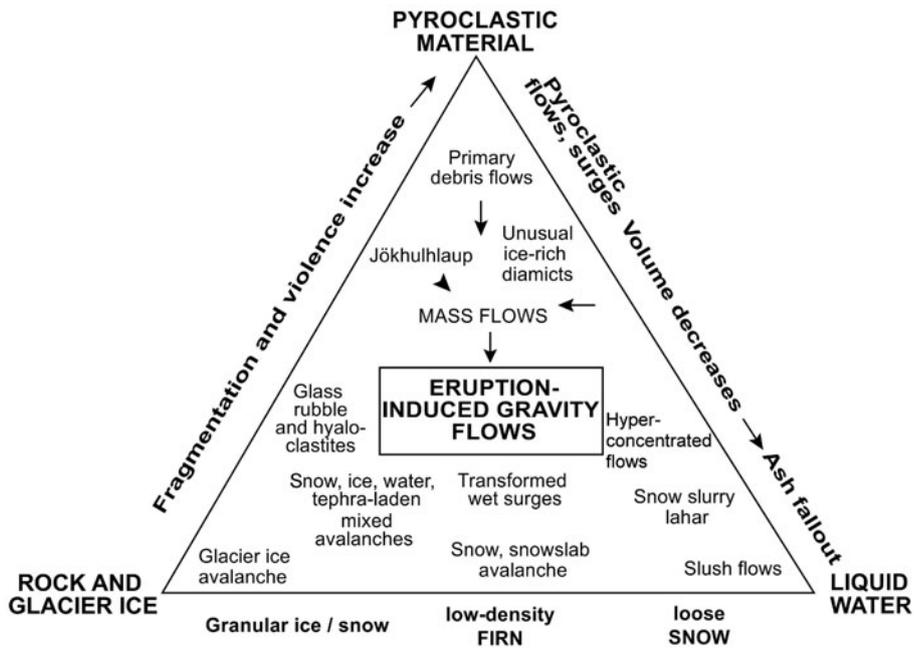
**Fig. 1.** Multiphase gravity flows and deposits linked to volcano–glacier interactions on composite cones. This ternary diagram (modified from Manville and others, 2000) is based on the Mt St Helens (1980), Nevado del Ruiz (1985), Mt Redoubt (1990), Mt Spurr (1992) and Ruapehu (1995) case studies.
