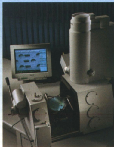
The new XL40 FEG SEM features a 150 mm motorized eucentric stage, conical end-lens and large chamber with full system automation and integrated image analysis.
