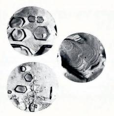
Figs. 2 and 3 (left). Microphotographs of shadowed replicas of etched ice crystals. The crystal in Fig. 2 and the grain on the left of Fig. 3 have faces perpendicular to the c-axis. The right hand grain in Fig. 3 has a face parallel to to the c-axis. Magnification ×13
