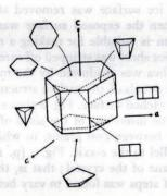
Fig. 1. Diagram to show the kinds of etch pits formed on ice
