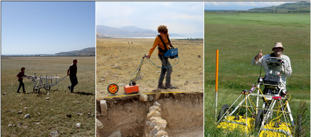
Figure 4. Geophysical methods in use at Artanish 9; left) magnetic gradiometry (2022); centre) GPR (GSSI SIR with single 400MHz antenna, 2022 & 2024); right) GPR (PulseEKKO Spidar bistatic system with two 250MHz antennas, 2023) (figure by B. Ullrich).
