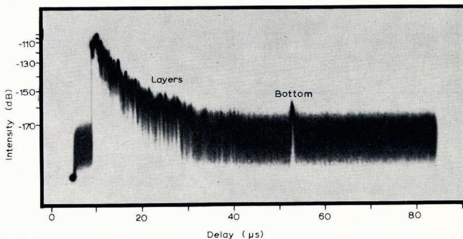
Fig. 6. A typical A-scope display showing layer echoes. The intensity scale is  $P_R/P_T$  in dB.
