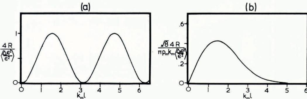
Fig. 5. The variation of the reflection coefficient  $R$  with layer thickness  $l$  for (a) a single layer and (b) multiple random layers.
