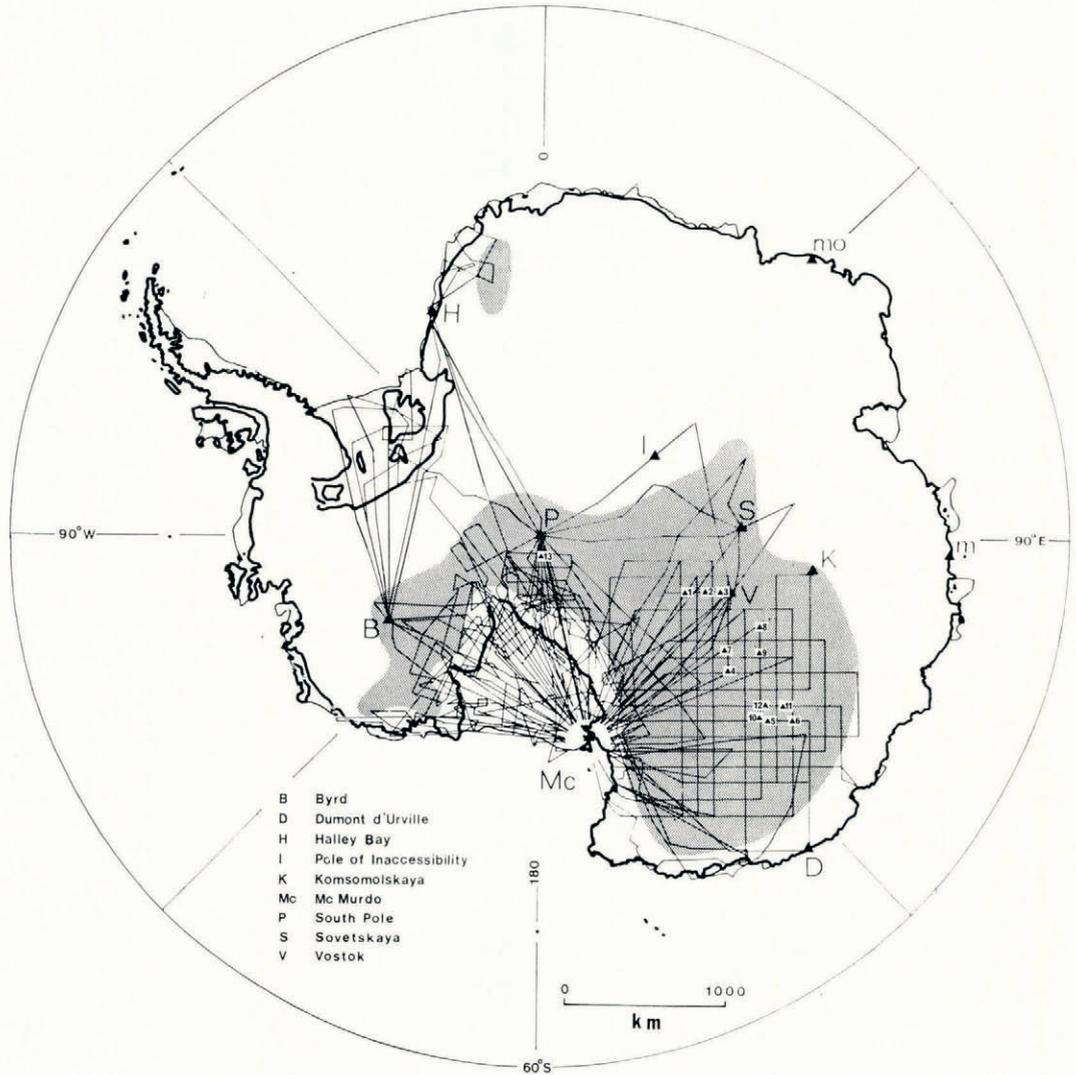
Fig. 1. The flight lines covered by the S.P.R.I.-N.S.F. surveys in the Antarctic and the geographical distribution of observed layer echoes (stipple). Measurements of the reflection coefficient of the layers and the attenuation per unit depth have been made at the numbered sites (Table I).
