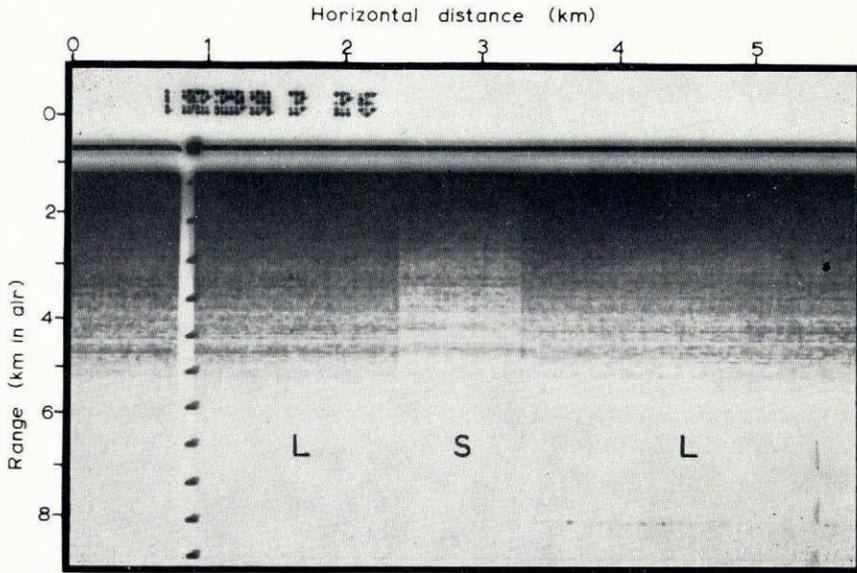
Fig. 7. Radio echo record showing a slight change in position of some of the layer echoes on alteration of pulse length;  $L \equiv 1 \mu\text{s}$ ,  $S \equiv 250 \text{ ns}$ .
