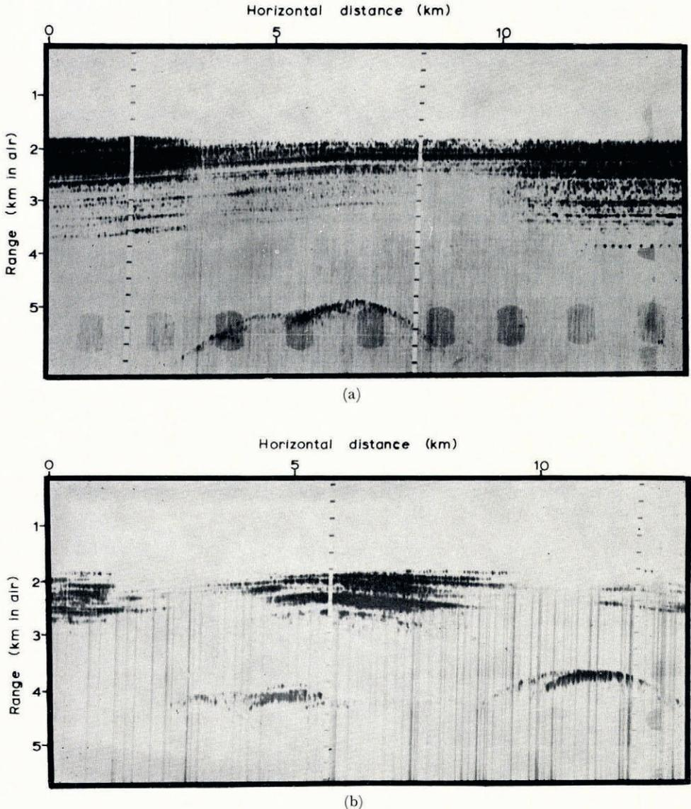
Fig. 10. Radio echo records showing weakening of the layer echoes over mountainous bedrock.
