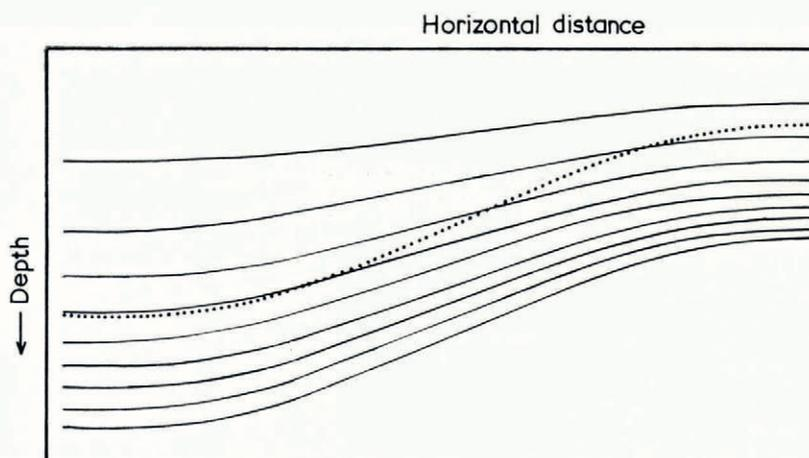
Fig. 9. Diagram showing a line of constant reflection coefficient (constant layer thickness) (dotted line) as the layered ice passes over mountainous bedrock.
