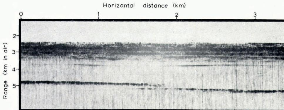
Fig. 8. Radio echo record showing fading layer echoes where the fading rates at different depths are unrelated.
