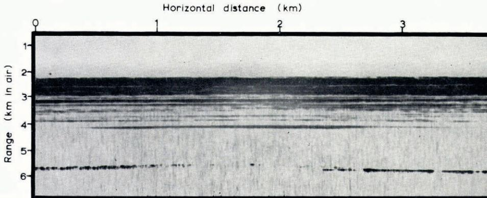
Fig. 3. Layer echoes showing the characteristic low fading rates (long fading length) and the characteristic vertical spacing.
