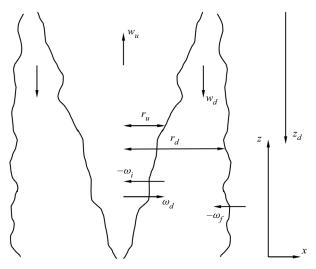
Figure 12. Fountain model BK00, with the arrows indicating the direction of variables.
