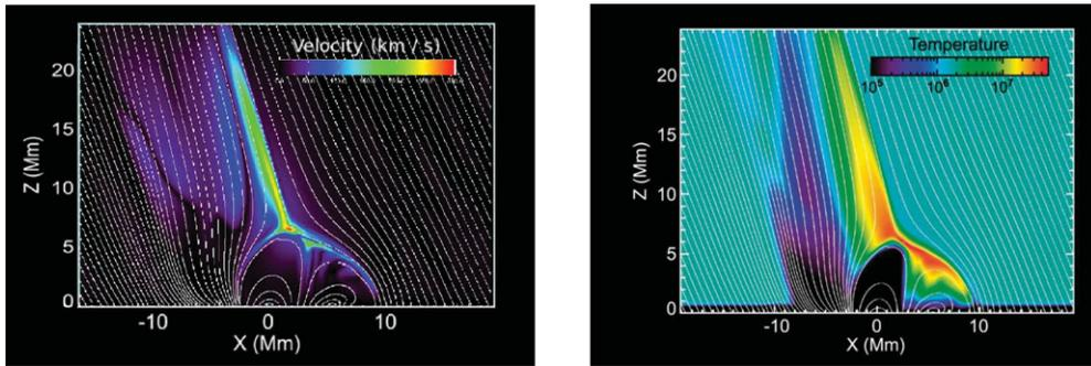
**Figure 5.** Velocity and temperature maps in a vertical cut of the three-dimensional experiment of Moreno-Insertis *et al.* (2008) around the time of peak jet activity
