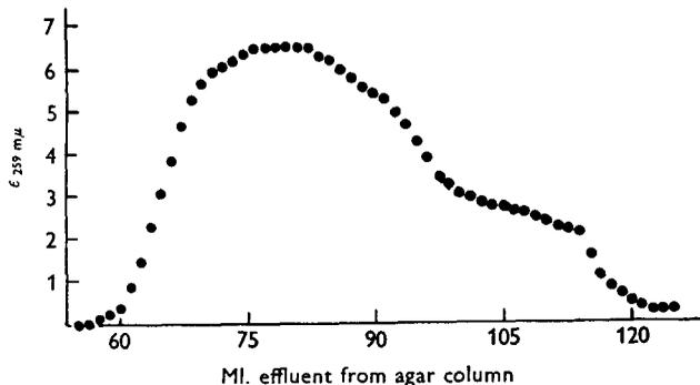
Fig. 11. Diffusion-filtration of high molecular deoxyribonucleic acid in a column of granulated 7% agar gel.
