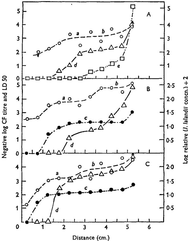
Fig. 3. Sedimentation of *S*<sub>10w</sub> RVF and MEF<sub>1</sub> poliovirus during 5 hr. at 33,000 r.p.m. in the presence of *J. lalandii* haemocyanin. Diagrams A, B and C refer to different experiments. For the preparation of the *S*<sub>10w</sub> RVF see text. The points refer to successive 0.5 cm. layers. Curves a, b—infectivity; curve c—complement fixation; curve d—relative haemocyanin concentration; curve e—infectivity titre of poliovirus.
