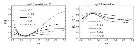
FIGURE 5. Reflection coefficient  $|R_p|$  and total energy  $|R_p|^2 + |T_p|^2$  against Kh when  $\mu = 1.2$ .
