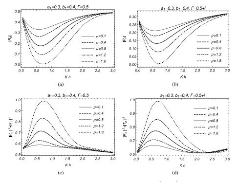
FIGURE 3. Reflection coefficient  $|R_p|$  and total energy  $|R_p|^2 + |T_p|^2$  against Kh.
