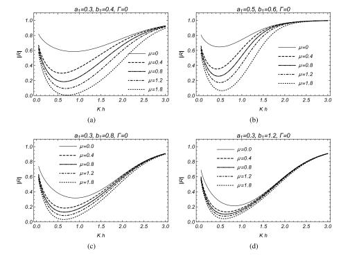
FIGURE 2. Reflection coefficient |R| against *Kh*.
