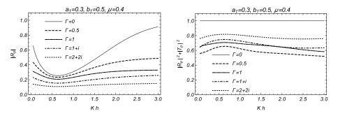
FIGURE 4. Reflection coefficient  $|R_p|$  and total energy  $|R_p|^2 + |T_p|^2$  against Kh when  $\mu = 0.4$ .
