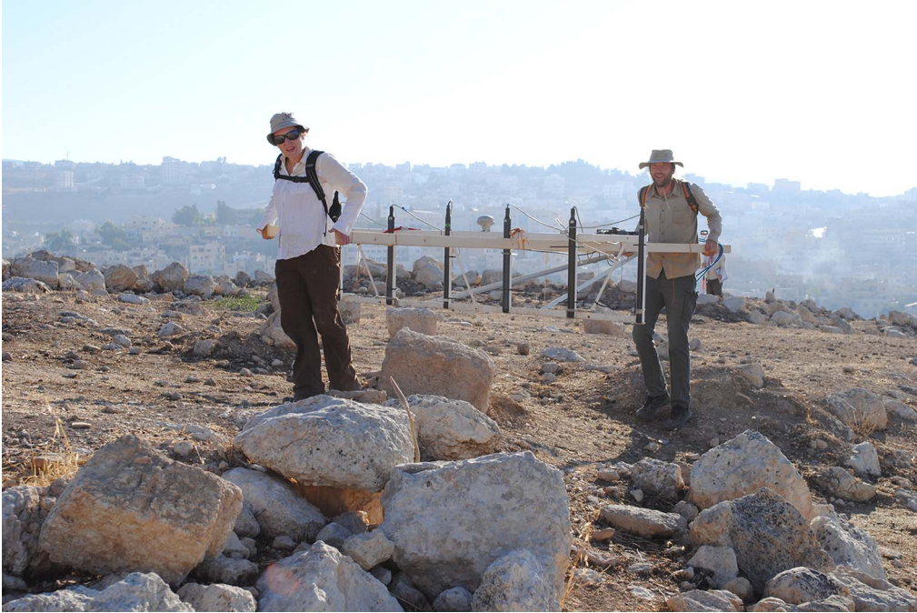
Figure 4. Fluxgate gradiometer in action in the Northwest Quarter (©Danish-German Jerash Northwest Quarter Project).
