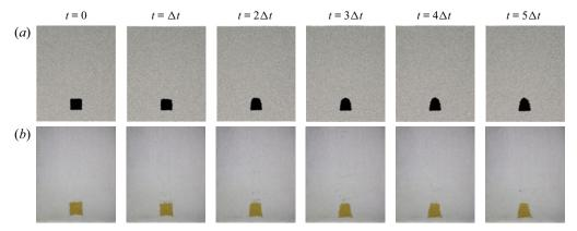
Figure 11. Time series of a stagnant cone. (a) Euler–Lagrange simulation of a cluster with  $d^* = 1.75$ ,  $\Delta \rho^* = 1.2$  and  $\Delta t = 4$  s. (b) Experiment (table 3 F) with  $d^* = 1.57$ ,  $\Delta \rho^* = 1.16$  and  $\Delta t = 60$  s.
