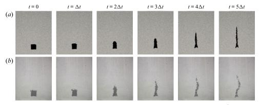
Figure 8. Time series of a rising finger. (a) Euler–Lagrange simulation of a cluster with  $d^* = 1.75$ ,  $\Delta \rho^* = 0.9$  and  $\Delta t = 2$  s. (b) Experiment (table 3 G) with  $d^* = 1.8$ ,  $\Delta \rho^* = 0.9$  and  $\Delta t = 8$  s.
