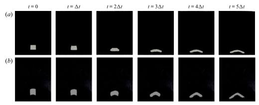
Figure 10. Time series of a sinking droplet. (a) Euler–Lagrange simulation of a cluster with  $d^* = 0.75$ ,  $\Delta \rho^* = 2.38$  and  $\Delta t = 1$  s. (b) Experiment (table 3 J) with  $d^* = 0.72$ ,  $\Delta \rho^* = 2.42$  and  $\Delta t = 2$  s.
