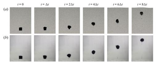
Figure 5. Time series of a rising bubble as obtained by (a) simulations and (b) experiments (table 3 A). Both rows show a cluster with  $d^* = 2$  and  $\Delta \rho^* = 0.9$ . Time steps of the images are  $\Delta t = 0.5$  s for simulations and 1 s for experiments.
