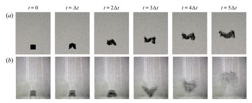
Figure 9. Time series of a disintegrating bubble. (a) Euler–Lagrange simulation of a cluster with  $d^* = 0.5$ ,  $\Delta \rho^* = 1.1$  and  $\Delta t = 2.4$  s. (b) Experiment (table 3 H) with  $d^* = 0.38$ ,  $\Delta \rho^* = 1.11$  and  $\Delta t = 6$  s. In the experiment, cluster particles are dark grey, bulk particles are light grey, whereas emerging gas bubbles are black.
