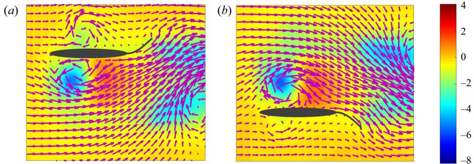
Figure 42. Changed tail length:  $\kappa h = 1.5$ ,  $\gamma = 0.1$ , aft-tail length  $L_t = 0.38c$ . Pressure coefficient ( $C_p$ ) contours during the end of (a) upstroke ( $t/T = 110.25$ ), and (b) downstroke ( $t/T = 110.75$ ).
