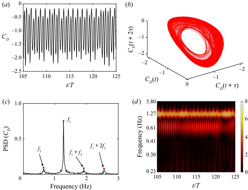
Figure 19. For  $\kappa h = 1.2$ , rigid tail, time series analysis of  $C_D$  indicates quasi-periodic dynamics: (a) time history, (b) reconstructed phase portrait, (c) frequency spectra, and (d) wavelet transform.
