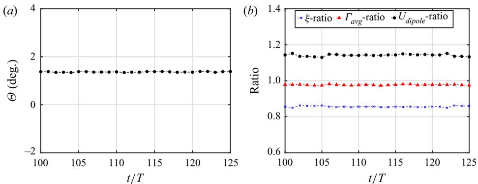
Figure 40. Changed tail length:  $\kappa h = 1.5$ ,  $\gamma = 0.1$ , aft-tail length  $L_t = 0.38c$ . (a) Wake deflection angle and (b) quantitative measures associated with the vortex system. Dominant effect of the upward deflecting vortex couple  $A-B$  results in a positive deflection angle.
