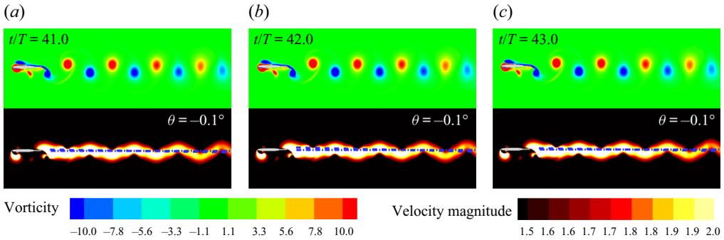
Figure 14. For  $\kappa h = 1.0$ , rigid tail: instantaneous vorticity (top) and velocity magnitude (bottom) contours depicting a reverse Kármán wake with mild downward deflection. Note that the same contour levels have been used throughout the paper for all the vorticity and velocity contour plots, and are therefore not repeated hereafter.
