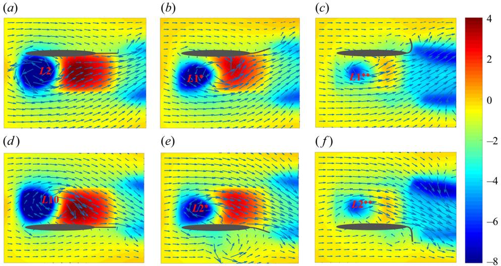
Figure 36. For  $\kappa h = 1.5$ , comparison of pressure coefficient ( $C_p$ ) contours during the end of (a–c) upstroke ( $t/T = 110.25$ ) and (d–f) downstroke ( $t/T = 110.75$ ), for (a,d) rigid tail, (b,e) flexibility level I, and (c,f) flexibility level II. Lengths of arrows indicate the magnitude of the velocity vector field.
