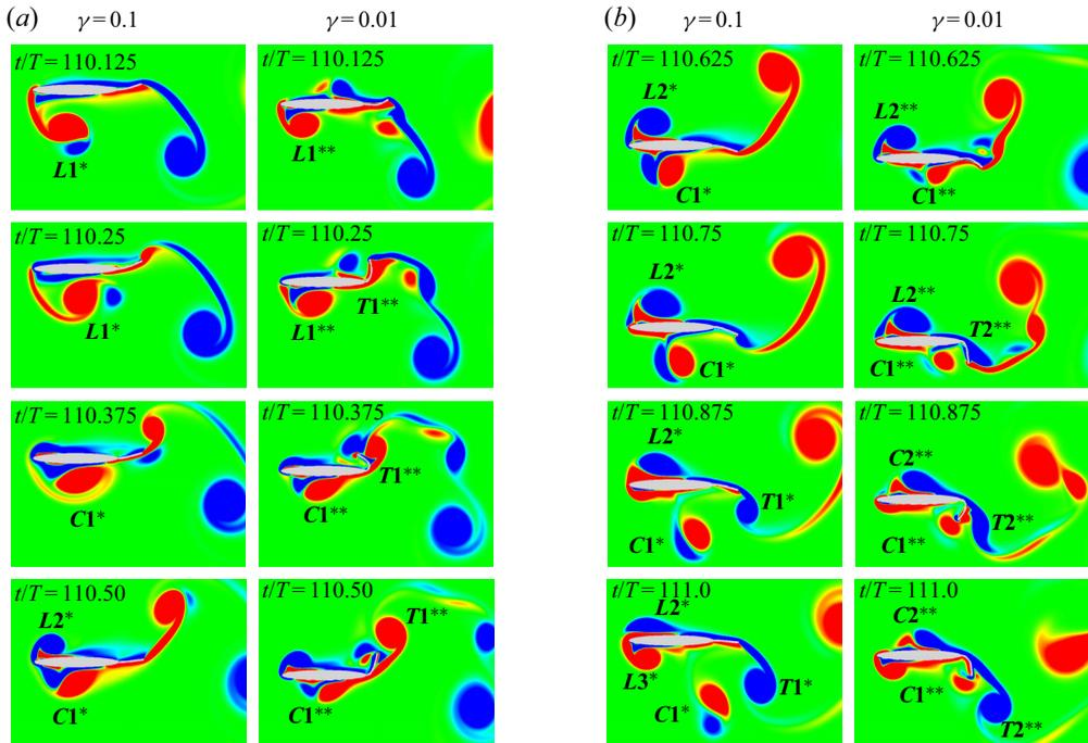
Figure 34. For  $kh = 1.5$ , comparison of near-field vortex interactions at the 111th cycle: (a) first half-cycle, (b) second half-cycle; each left-hand column shows flexibility level I, and each right-hand column shows flexibility level II.
