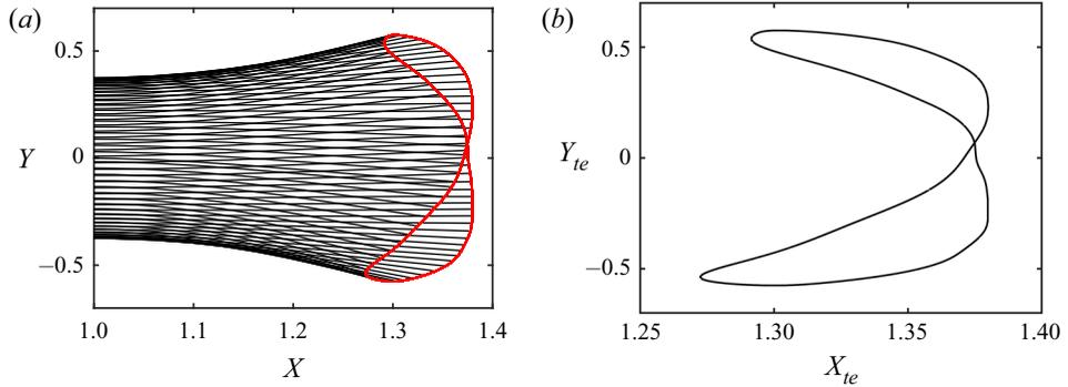
Figure 41. Changed tail length:  $\kappa h = 1.5$ ,  $\gamma = 0.1$ , aft-tail length  $L_t = 0.38c$ , (a) Deflection envelopes, mode shape structure. (b) Phase plot of the tail-tip of the flexible tail.
