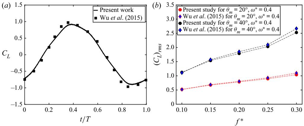
Figure 10. (a) Comparison of lift coefficient  $C_L$  for  $\theta_m = 20^\circ$ ,  $m_t^* = 5$ ,  $\omega^* = 0.4$  and  $f^* = 0.15$ . (b) Root-mean-square values of lift coefficient  $(C_L)_{rms}$  with the work of Wu *et al.* (2015) at  $Re = 1100$ . Parametric symbols follow the definitions given by Wu *et al.* (2015).
