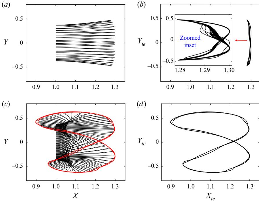
Figure 35. For  $\kappa h = 1.5$ , deflection envelopes and phase portraits for the tip displacement of the flexible tail for flexibility level I (a,b) and flexibility level II (c,d). (a) Mode shape structure for flexibility level I. (b) Phase plot of the free end of the trailing edge for flexibility level I. (c) Mode shape structure for flexibility level II. (d) Phase plot of the free end of the trailing edge for flexibility level II.
