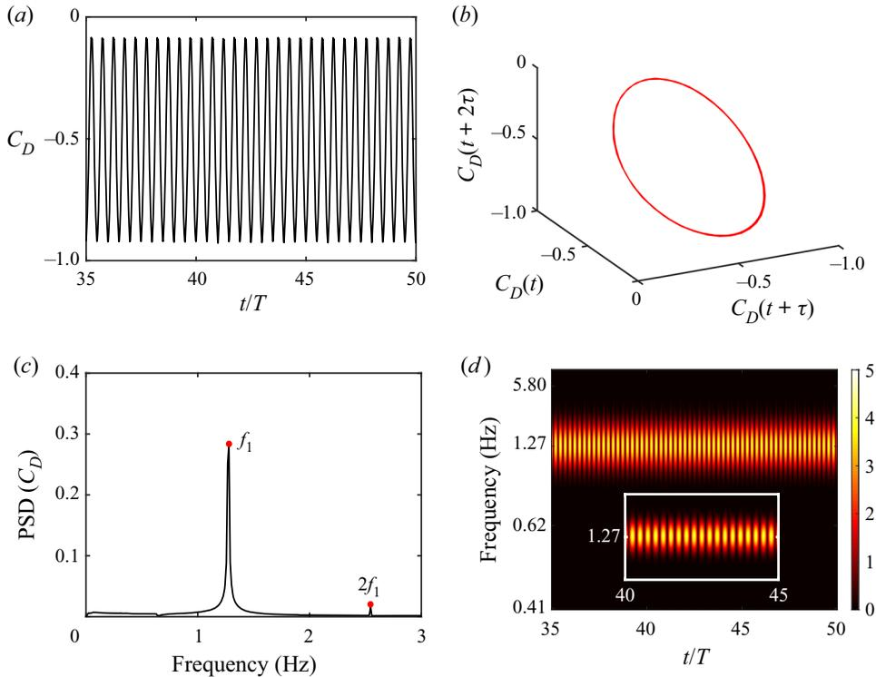
Figure 16. For  $\kappa h = 1.0$ , rigid tail, time series analysis of  $C_D$  indicates periodic dynamics: (a) time history, (b) reconstructed phase portrait, (c) frequency spectra (where PSD denotes power spectral density), and (d) wavelet transform.
