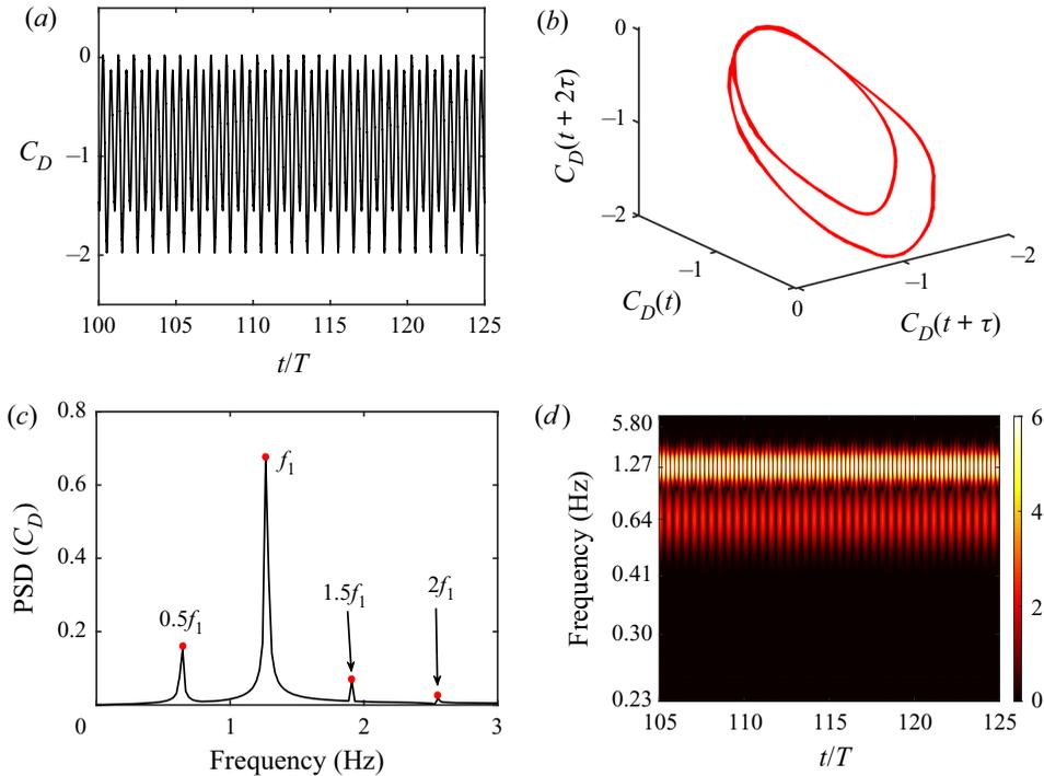
Figure 37. Changed tail length:  $\kappa h = 1.5$ ,  $\gamma = 0.1$ , aft-tail length  $L_t = 0.38c$ . Time series analysis of  $C_D$  indicates periodic dynamics: (a) time history, (b) reconstructed phase portrait, (c) frequency spectra, and (d) wavelet transform.
