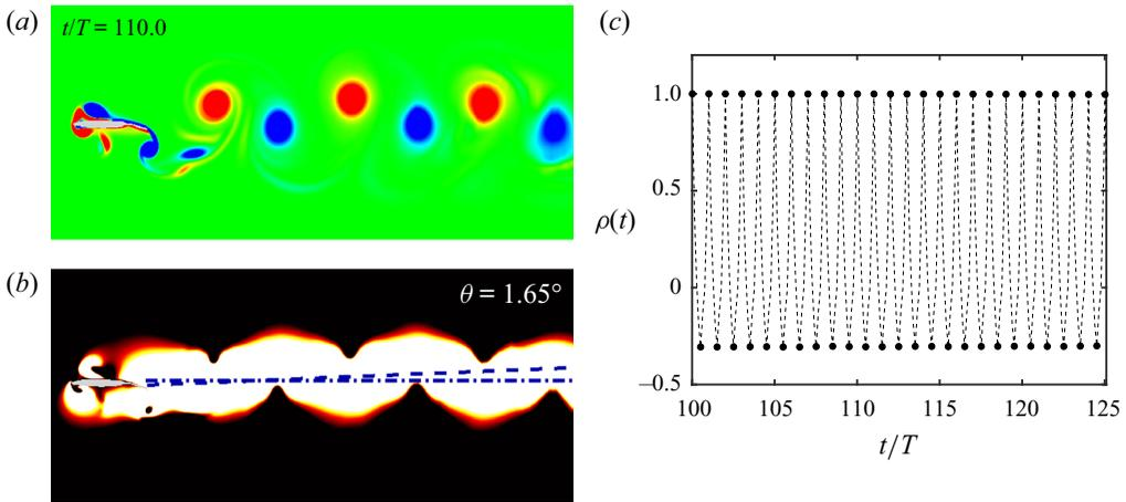
Figure 39. Changed tail length:  $\kappa h = 1.5$ ,  $\gamma = 0.1$ , aft-tail length  $L_t = 0.38c$ . (a) Instantaneous vorticity and (b) velocity magnitude, contours depicting reverse Kármán wake with mild upward deflection; and (c) vorticity correlation.
