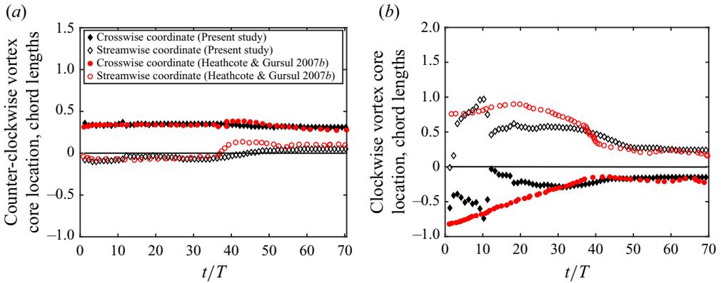
Figure 12. Comparison of vortex core location in chord lengths obtained from the present simulation and the experimental work of Heathcote & Gursul (2007b);  $h = 0.194$  and  $b/c = 1.13 \times 10^{-3}$ . Note that the parametric symbols follow the definitions given by Heathcote & Gursul (2007b), equivalent to  $\gamma = 0.496$ : (a) counter-clockwise vortex, and (b) clockwise vortex.
