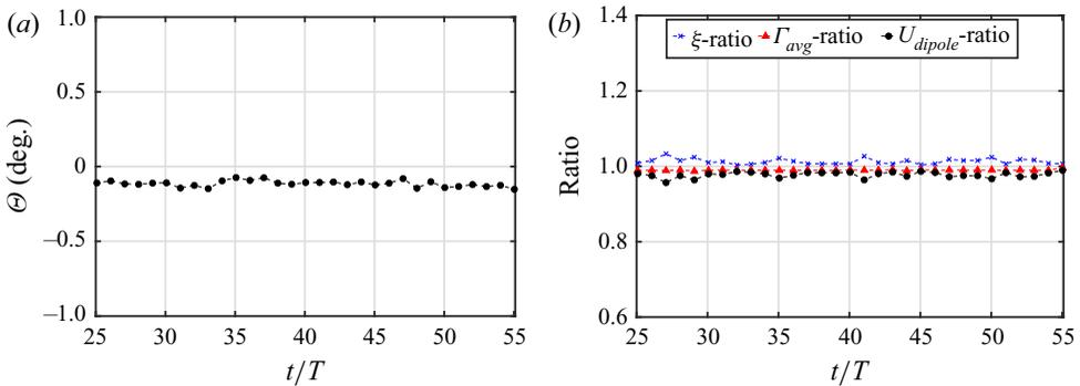
Figure 15. For  $\kappa h = 1.0$ , rigid tail: (a) wake deflection angle, (b) quantitative measures associated with the vortex system. Dominant effect of the downward deflecting vortex couple  $B-C$  results in negative deflecting angle.
