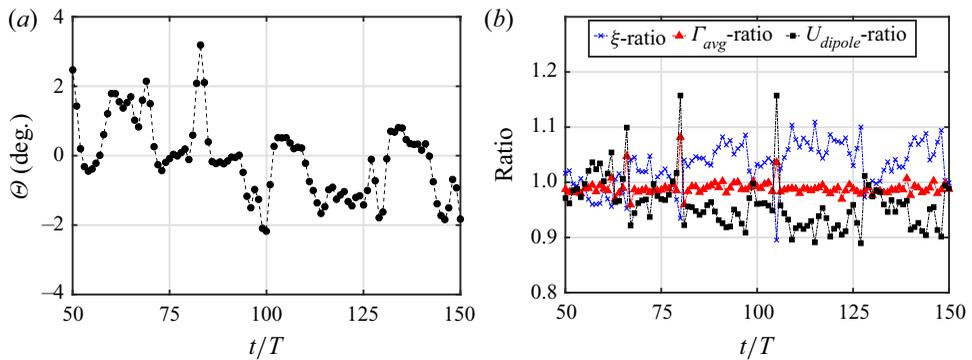
Figure 18. For  $\kappa h = 1.2$ , rigid tail: (a) wake deflection angle, (b) quantitative measures associated with the vortex system. Alternate dominance of the upward and downward deflecting vortex couples leads to jet-switching.
