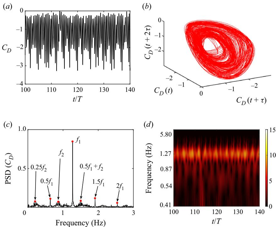
Figure 26. For  $\kappa h = 1.5$ , flexibility level I, time series analysis of  $C_D$  indicates quasi-periodic dynamics: (a) time history, (b) reconstructed phase portrait, (c) frequency spectra, and (d) wavelet transform.
