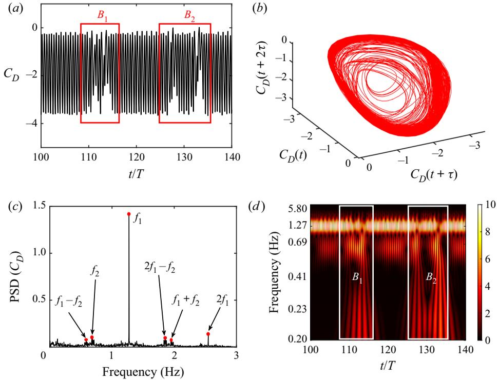
Figure 21. For  $\kappa h = 1.5$ , rigid tail, time series analysis of  $C_D$  during type-II intermittency: (a) time history, (b) reconstructed phase portrait, (c) frequency spectra, and (d) wavelet transform.
