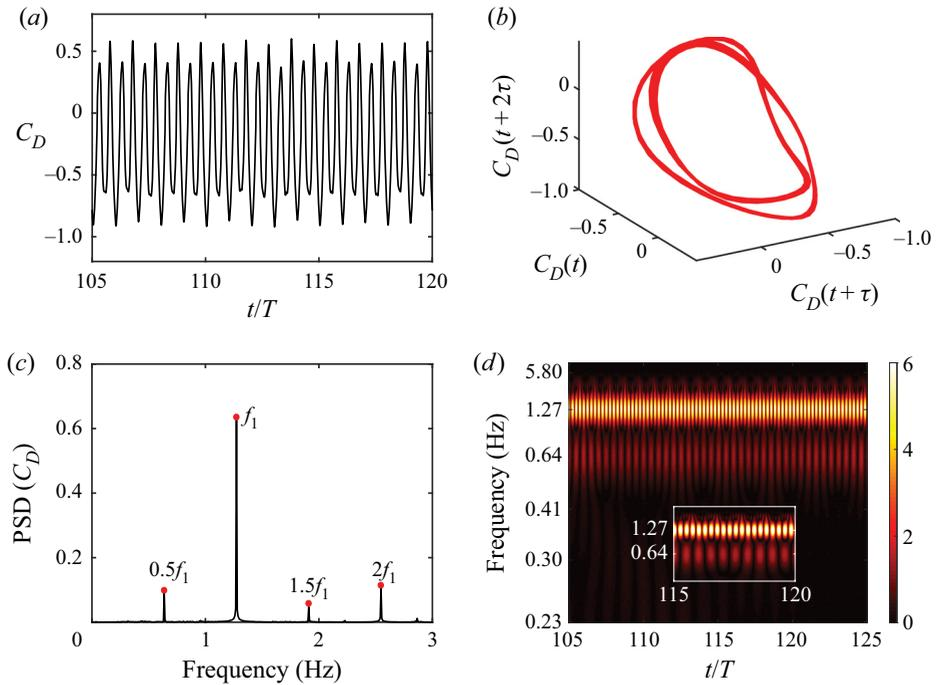
Figure 29. For  $\kappa h = 1.5$ , flexibility level II, time series analysis of  $C_D$  indicates periodic dynamics: (a) time history, (b) reconstructed phase portrait, (c) frequency spectra, and (d) wavelet transform.
