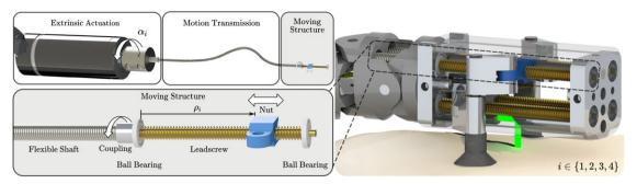
**Figure 4.** The actuation concept for the miniature parallel robot: Flexible shafts are transmitting the rotation  $\alpha_i$  from the externally placed electrical motors to the rotation of the leadscrews inside the end effector. These leadscrews then transfer the rotary motion of the flexible shafts into linear movements of nuts  $\rho_i$ , that is, the prismatic actuators. The miniature robot houses four such prismatic actuators.
