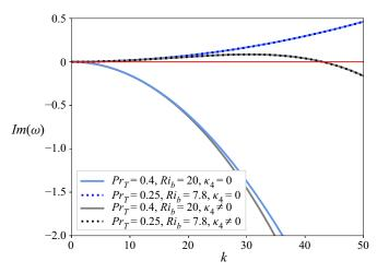
Figure 9. Growth rate as a function of the wavenumber k for various sets of parameters and with or without hyperdiffusion  $\kappa_4$ . The red horizontal line corresponds to  $Im(\omega) = 0$ . The blue curves (corresponding to  $\kappa_4 = 0$ ) unveil an 'ultraviolet catastrophe' of unbounded growth at small scales (i.e. large vertical wavenumbers k).
