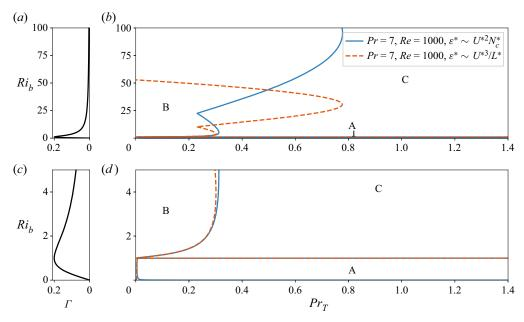
Figure 8. (a-d) Range of bulk Richardson numbers  $Ri_b$  and turbulent Prandtl numbers  $Pr_T$  prone to staircase formation for Pr = 7 and Re = 1000, using parameterisation (2.11) of  $\Gamma$  with p = 1 (depicted in a,c) for the different scalings for the dissipation rate of turbulent kinetic energy  $\epsilon^*$  discussed in § 2.2. A zoom-in of region A is shown in (c,d).
