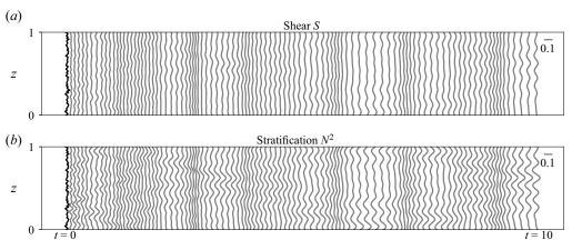
Figure 15. Evolution of shear and stratification profiles for case O with  $Ri_b = 7.8$ ,  $Pr_T = 0.25$ , Pr = 7 and Re = 1000. The black lines correspond to the initially disturbed profiles. The horizontal axis is time and each profile is separated by a 0.1 dimensionless time unit. We use the lower value of  $\kappa_4 = 10^{-7}$ .
