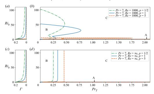
Figure 6. (a,b) Range of bulk Richardson numbers  $Ri_b$  and turbulent Prandtl numbers  $Pr_T$  prone to staircase formation for Pr = 7 and Re = 1000, using parameterisation (2.11) of  $\Gamma$  with various power laws p (depicted in a,c). (c,d) Same as (a,b) but with  $Re = \infty$ . Note that the behaviour of  $\Gamma$  at small  $Ri_b$  is independent of p. Hence, region A is similar to the one depicted in figure 4.
