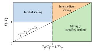
Figure 2. Scaling used depending on the relative size of  $T_b^*$  (buoyancy time scale),  $T_S^*$  (shear time scale) and  $T_T^*$  (turbulent time scale). The solid horizontal line corresponds to  $T_T^*/T_S^*=1$ . The dashed vertical line corresponds to  $T_D^*/T_S^*=1$ .
