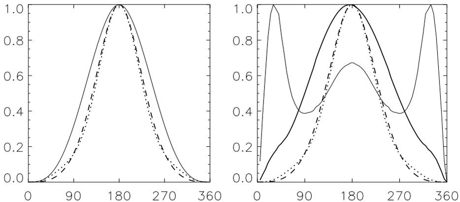
**Figure 2.** (a) Orbital reflected light curves of three uniform planets observed at  $i = 90$  deg. with and different scattering laws; Lambertian (solid line), single RS (dotted line) and a model of Mercury (dashed line) (Warell 2004). (b) Light curves of “smooth” (ocean) planets (solid lines) with 0% (thin) and 38% (thick) cloud cover compared to RS and Mercury models. All curves have been normalized.
