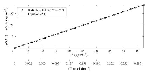
FIGURE 8. Density difference between aqueous solutions of KMnO<sub>4</sub> and water (symbols) as a function of KMnO<sub>4</sub> concentration at constant temperature ( $T^* = 23 \,^{\circ}\text{C}$ ,  $\rho^*(0) = 997.54 \text{ kg m}^{-3}$ ). The linear function defined by (2.1) (solid line) approximates very well the correlation proposed by Novotný & Söhnel (1988) (symbols) in the range of values of interest.
