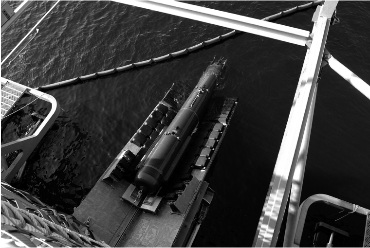
Figure 1.20 The Seahorse-class Autonomous Underwater Vehicle is moved into position for launch. (credit: Stocktrek Images / Getty Images)
