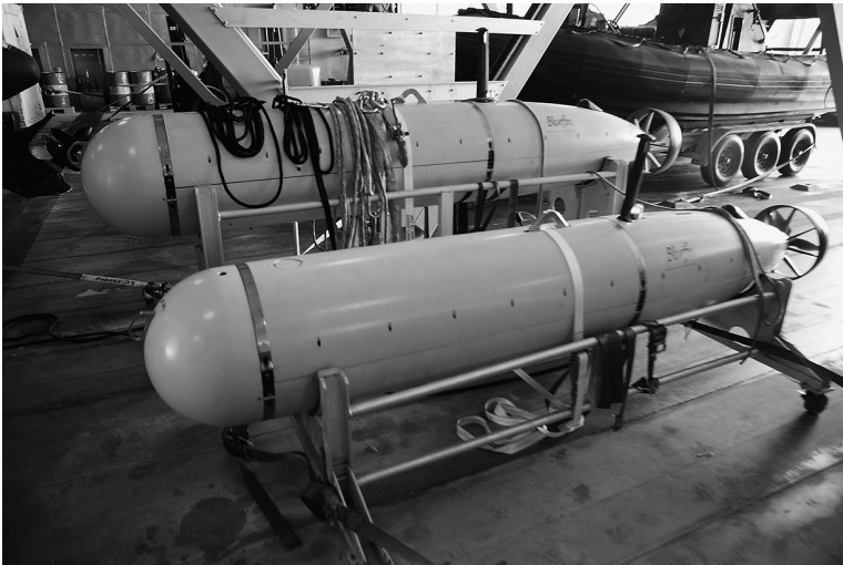
Figure 1.21 AUV for underwater surveillance. (credit: Marco Garcia / Stringer / Getty Images News)
