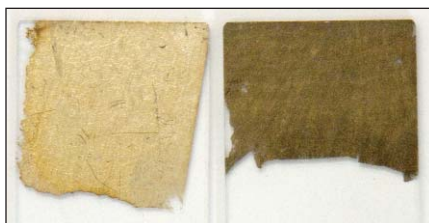
Figure 2. Nanoporous gold on glass microscope slides. Note the unusually dark copper color of the slide on the right, which had been dealloyed for a much longer time than the sample on the left.
