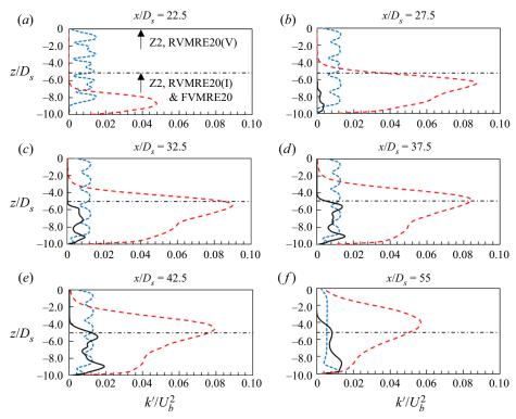
Figure 21. (a-f) Vertical distributions of the dimensionless width-averaged TKE  $k'/U_b^2$  within and downstream of the vegetation zone for different  $x/D_s$ . The meanings of the different types of lines in the figure are the same as in figure 16.
