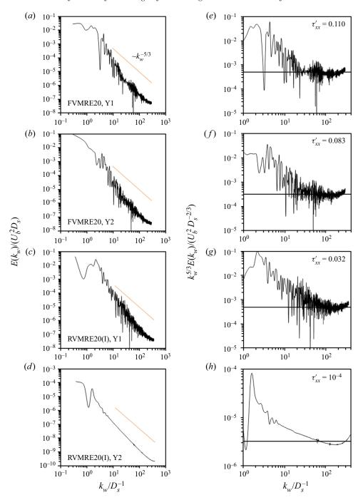
Figure 19. (a-d) Energy spectra  $E(k_w)$  and (e-h) estimations of the TKE dissipation rate  $\varepsilon$  in flow with stationary (RVMRE20(I) case) and moving (FVMRE20 case) vegetation. Here  $\tau'_{xx}$  represents the streamwise Reynolds normal stress, i.e.  $\tau'_{xx} = \overline{u'u'}/U_b^2$ .
