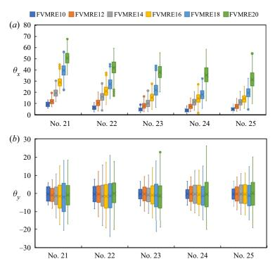
Figure 13. Movement of five plants (numbers 21–25) under different flow velocities. Distributions of (a) the streamwise swaying amplitude  $\theta_x$  and (b) the spanwise swaying amplitude  $\theta_y$  of the top of the plants. The six colours represent six cases with Reynolds numbers varying from 10 000 to 20 000, corresponding to the FVMRE10–FVMRE20 cases. The symbols used in the figure are same as in figure 12.
