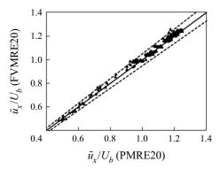
Figure 7. Comparison of the dimensionless time-averaged streamwise velocity  $\bar{u}_x/U_b$  of flow at all 192 ADV measuring points in the PMRE20 case and the computed value of  $\bar{u}_x/U_b$  at the corresponding positions in the FVMRE20 case. The solid line is the y=x auxiliary line, representing the zero error. The two dotted lines are y=1.05x and y=0.95x auxiliary lines, representing 5% error.
