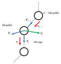
Figure 3. Dynamics of the *l*th pellet and its adjacent pellets. The blue arrows represent the force vectors, the red arrows represent the unit vectors in the direction of the ropes, and the green arrows represent the velocity vectors. The physical parameters represented by the notation in the figure are explained in § 2.3.
