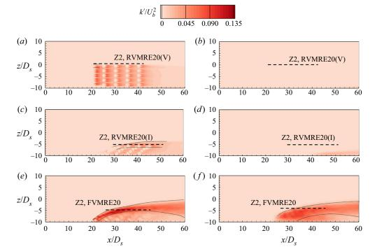
Figure 20. Dimensionless TKE structures  $k'/U_b^2$  simulated in (a) the RVMRE20(V) case on the Y1 plane with  $y/D_s=0$ , (b) the RVMRE20(V) case on the Y2 plane with  $y/D_s=2.5$ , (c) the RVMRE20(I) case on the Y1 plane, (d) the RVMRE20(I) case on the Y2 plane, (e) the FVMRE20 case on the Y1 plane and (f) the FVMRE20 case on the Y2 plane.
