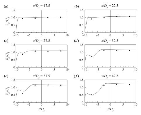
Figure 8. (a-f) Vertical distributions of the dimensionless time-averaged streamwise velocity  $\bar{u}_x/U_b$  on the  $y/D_s = 2.5$  plane for different  $x/D_s$ . The triangle symbols represent the measured results of the physical model study. The solid lines represent the simulation results of the FVMRE20 case.
