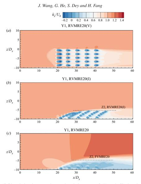
Figure 15. Dimensionless time-averaged streamwise velocity structures  $\bar{u}_x/U_b$  on the Y1 plane simulated numerically in the (a) RVMRE20(V) (vertical rigid vegetation with  $Re = 20\,000$ ), (b) RVMRE20(I) (inclined rigid vegetation with  $Re = 20\,000$ ) and (c) FVMRE20 (flexible vegetation with  $Re = 20\,000$ ) cases. Owing to vegetation movement, the characteristic location Z2 (that is, the flow-vegetation interface) is not a fixed plane in (b and c).
