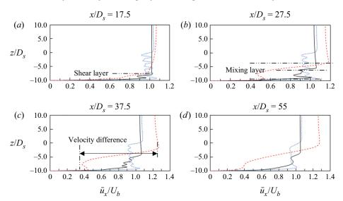
Figure 16. (a-d) Vertical distributions of the dimensionless width-averaged streamwise velocity  $\bar{u}_x/U_b$  within and downstream of the vegetation zone for different  $x/D_s$ . The solid lines represent the simulation results of the RVMRE20(I) case, the blue dotted lines represent the simulation results of the RVMRE20(V) case and the red broken lines represent the simulation results of the FVMRE20 case.
