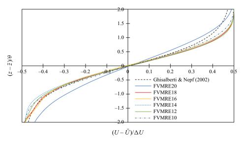
Figure 9. Time-averaged flow velocity distributions for the FVMRE20–FVMRE10 cases. The comparison between the simulated velocity profiles and the hyperbolic tangent flow velocity curve (Ghisalberti & Nepf 2002) is satisfactory.
