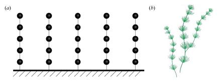
Figure 2. (a) Shape of the plants in the numerical model. The fine lines in the figure do not exist in the numerical model, but are realised by constraining the relative motion between the pellets. (b) C. demersum. By varying the number and diameter of the pellets contained in a single plant in (a), different shape characteristics of the plants can be simulated.
