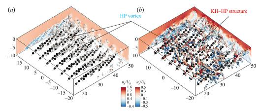
Figure 18. Vortex structure of flow in the vegetation zone obtained from (a) the RVMRE20(I) and (b) the FVMRE20 cases. The vortex structure in the figure is represented by the iso surface of pressure fluctuation. The colour of the background flow field indicates the instantaneous velocity. The colour of the pressure pulsation iso surface indicates the velocity fluctuation.
