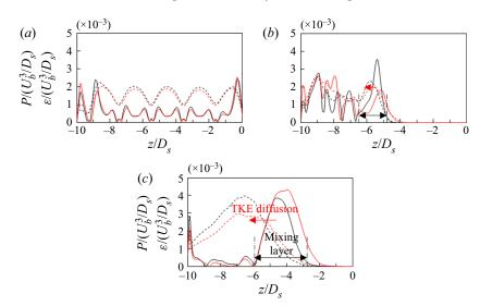
Figure 22. Vertical distributions of the dimensionless width-averaged TKE production rate  $P/(U_b^3 D_s)$  (solid lines) and the TKE dissipation rate (dotted lines) within and downstream of the vegetation zone in (a) the RVMRE20(V) case, (b) the RVMRE20(I) case and (c) the FVMRE20 case. The black lines represent the simulation results on the  $x/D_s = 37.5$  section, and the red lines represent the simulation results on the  $x/D_s = 42.5$  section.
