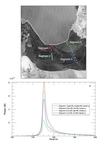
**Fig. 5.** (a) Segments 1–4 over the first-year sea-ice area (bounded by white dotted line) overlaid upon a TerraSAR-X radar image from 28 November 2013. TerraSAR-X image (courtesy DLR (German Aerospace Center)). (b) Mean waveforms from these segments plotted as power for multiple sea-ice surface conditions with variable geometric roughness (GR), radar roughness (RR) and snow depth  $(s_h)$ .
