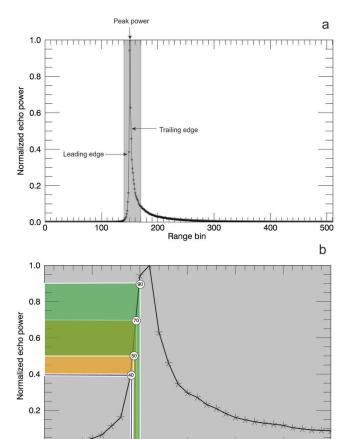
**Fig. 2.** (a) Typical CryoSat-2 SIN mode waveform over snow-covered sea ice in McMurdo Sound with labelling of characteristics mentioned in the text. (b) An expanded view of the outlined grey area in (a) from range bins 140–170 (1 bin = 0.234 m) and the expected retracking points on the leading edge for the techniques described here: *ESAL2* (40–70% orange), *WfF* (50–90% green) and *TFMRA40* (40% blue).
