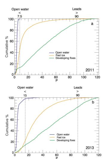
**Fig. 7.** Surface type discrimination as indicated by Level 2 parameter peakiness (*P*) displayed as a cumulative percentage. Surface types, open water, fast ice and developing floes are displayed for 2011 (a) and 2013 (b). In 2011, surface conditions made the discrimination of open water and fast ice more difficult. This resulted in a change in the thresholds between the years. The expected inclusion of sea ice in the open-water surface type is indicated by the percentage overlaps.
