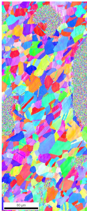
FIG. 1. Inverse pole figure revealing grain boundary orientations.
