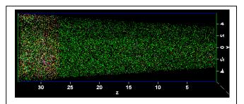
Figure 3. 3-D APT reconstruction showing distribution of carbon moieties of epoxy resin embedded sample.
