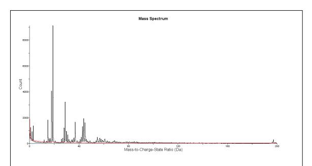
Figure 2. Atom Probe mass spectrum of an epoxy resin embedded sample. Peaks correspond to different C, N and O moieties. Implanted Ga is not detected.
