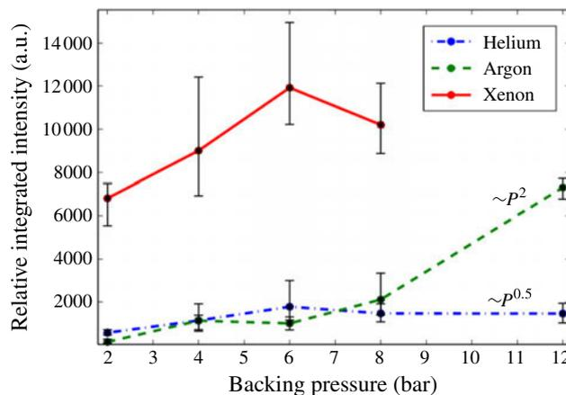
**Figure 4.** Comparison of the pressure dependence of the 25th harmonic at  $6.5 \times 10^{13} \text{ W cm}^{-2}$  intensity in He, Ar, and Xe.
