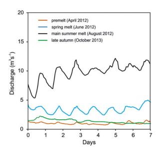
**Fig. 4.** Flow in the meltwater river at Virkisá bridge for four different weeks throughout the year, demonstrating the magnitude of the impact of the summer melt on river flow. During each period (and for at least 3 d prior) there was negligible precipitation.
