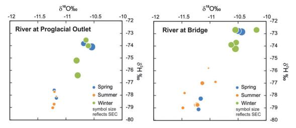
**Fig. 8.** Stable isotopes  $\delta^2 H$  and  $\delta^{18} O$ , and relative SEC in river samples collected at (a) the proglacial outlet and (b) the gauging station at Virkisá bridge (see Figs 1 and 2 for locations). Repeat wade gauging of flow at these two locations indicated flow to be similar to within 10%.
