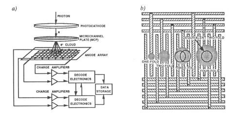
FIGURE 1. a) Block diagram of the MAMA detector operation, b) an illustration of two sets of interleaved anodes with different sized electron clouds.
