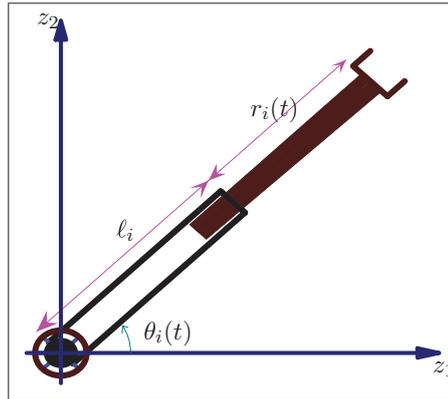
Fig. 11. Schematic representation of the  $i$ th planar (RP) manipulator in the  $z_1z_2$  plane. (Adopted from<sup>15</sup>)
