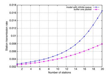
FIGURE 1. Computation of  $\tau(M)$  with and without buffer.
