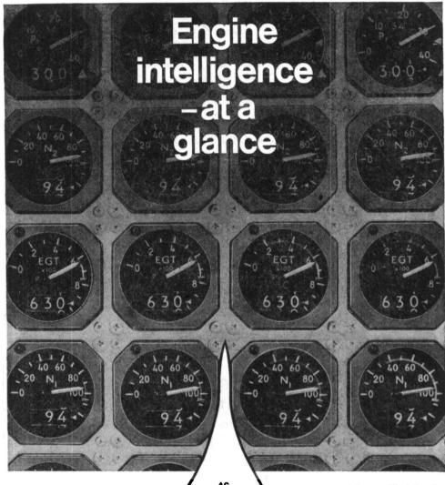
Designed for rapid, high accuracy scanning of engine parameters, these new counter/pointer engine indicators form a compact modular instrument package.
