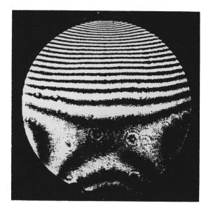
bending caused by any combination of cable tensions is given simply by a linear superposition of the 24 individual contributions. Similarly, if a given bending displacement is desired, then the combination of cable tensions that best reproduces it can be determined analytically by the method of least squares, once the influence function is known.
