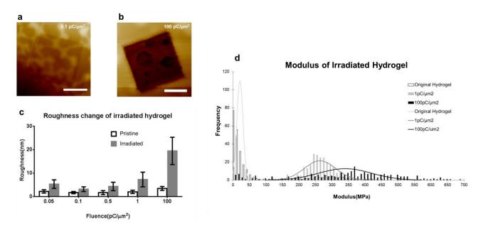
**Figure 1.** AFM images (top view) of surface morphology after ion milling (Ga<sup>+</sup>, 30 kV) with ion fluence (a) 0.1 pC/ $\mu$ m<sup>2</sup> and (b) 100 pC/ $\mu$ m<sup>2</sup>. (c) The corresponding numerical values of surface roughness of pristine hydrogel and after ion irradiation with increasing ion fluence. (Scale bar: 5  $\mu$ m) (d) Modulus of hydrogel before and after the ion beam irradiation.
