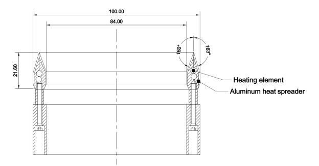
Fig. 4. Cross section of the melting head, showing the two windings of the hotspring<sup>®</sup> coil heater molded into the aluminum heat spreader.
