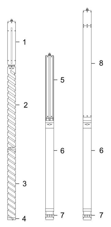
**Fig. 1.** Schematic of main components of the combined EM/thermal drill. Left: EM drill with 1. drive unit including motor and anti-torque system; 2. chips barrel with transport spiral; 3. core barrel with transport spiral; 4. cutting ring. Middle and right: TD with the two versions of the upper module with 5. upper module T; 6. core barrel; 7. melting head; 8. upper module C.
