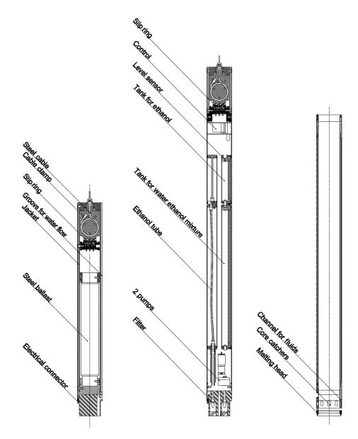
Fig. 2. Cross sections of the upper module T (left), the upper module C containing tanks for the antifreeze ethanol and the ethanol/water mixture (middle) and the core barrel with melting head (right).
