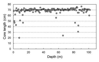
**Fig. 6.** Length of ice-core segments vs depth for EM (diamonds) and thermal drilling (squares) on Silvrettagletscher. Average length was 68 cm of the 70 cm targeted.
