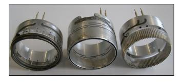
**Fig. 5.** Melting head with hotspring<sup>®</sup> coil heater of 100 mm outer diameter. Left: open heater; middle: simple aluminum heat spreader; right: aluminum crown with heat-spreader fins.
