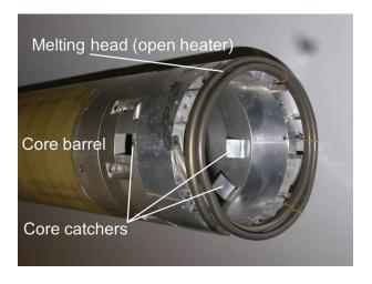
Fig. 3. Photo of the core barrel, including core catchers and melting head.
