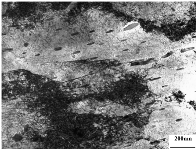
Fig. 1. TEM bright field images of martensite matrix and coarse phase for steel 1# (a), and for steel 2# (b).
