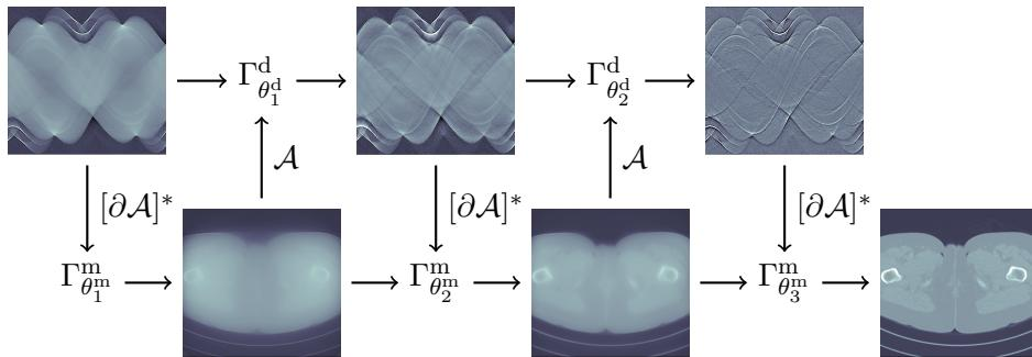
Figure 5.2. Learned iterative method in both model parameter and data spaces. Illustration of the operator obtained by unrolling the scheme in (5.14) for  $N = 3$  in the context of CT image reconstruction (Section 7.3.1).
