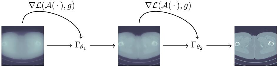
Figure 5.1. Learned iterative method in model parameter space. Illustration of the unrolled scheme in (5.11) for  $N = 2$  in the context of CT image reconstruction (Section 7.3.1). Each  $\Gamma_{\theta_k}: X \rightarrow X$  is a CNN,  $g \in X$  is the measured data, and  $f^0$  is an initial image, usually taken as zero.
