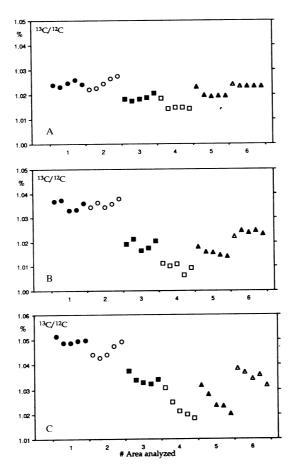
Fig 4. Examples of  $^{13}C^{3+}/^{12}C^{3+}$  ratios measured in the 6 analyzed areas of 3 targets during a run. The time between the measurements of 2 successive areas is close to 2 min; the time between 2 measurements in the same area is ca 1 hr.
