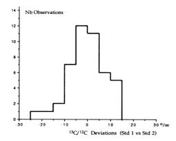
Fig 3. Histogram of the <sup>13</sup>C/<sup>12</sup>C deviations measured between the 2 Oxalic-I acid standards during the last 45 routine runs
