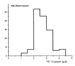
Fig 2. Histogram of the mean  $^{12}$ C- current output observed during the measurements of the last 150 targets prepared at Gif
