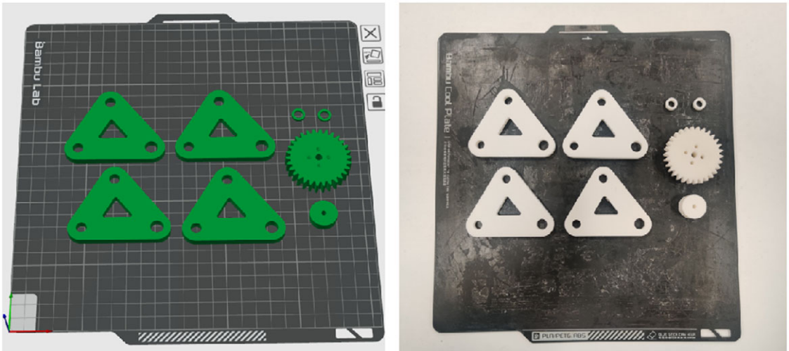
Figure 10. The links, gears and spacers are fabricated by 3D printing PLA.
