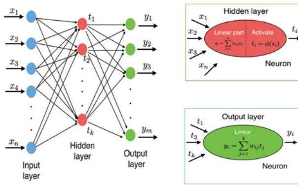
**Figure 1.** Typical architecture of an artificial neural network. The architecture of the ANN consists of an input layer, a hidden and an output layer of neurons. Each neuron connects the neurons in the next layer.
