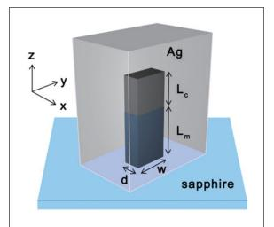
Figure 1. A schematic diagram of the surface plasmon polariton (SPP) cavity—a silver-covered dielectric nanorod consisting of a high-index material (dark grey) on top of a low index material (blue)—placed on a sapphire substrate.
