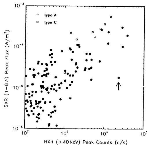
Fig. 3- Peak soft X-ray flux vs peak hard X-ray flux for 147 *Hinotori* flares. The 1981 October 15 flare is indicated by an arrow. Those flares showing clear spectral hardening over the peaks are classified as "type C" (7), while those with an extremely steep spectrum and small source size are classified as "type A" (3).
