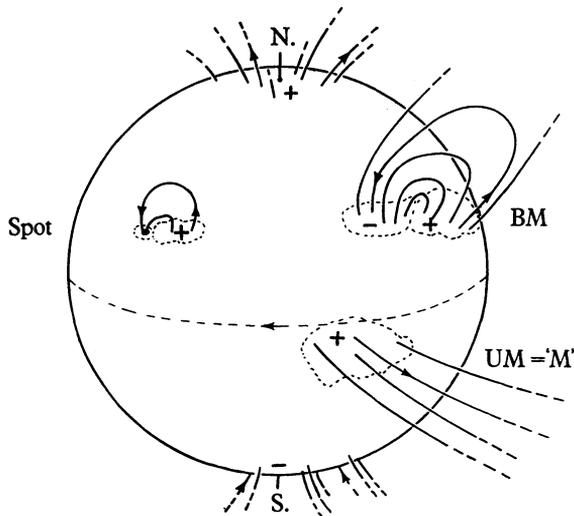
Fig. 2. Schematic representations of magnetic lines of force of (a) the general field, near the poles, (b) two BM regions, one with a spot, and (c) a UM region. Above UM regions, the lines of force are probably carried out to great distances by energetic corpuscular streams expelled from these regions; the lines of force presumably return through widespread areas in which the field is below the limit of detectability.
