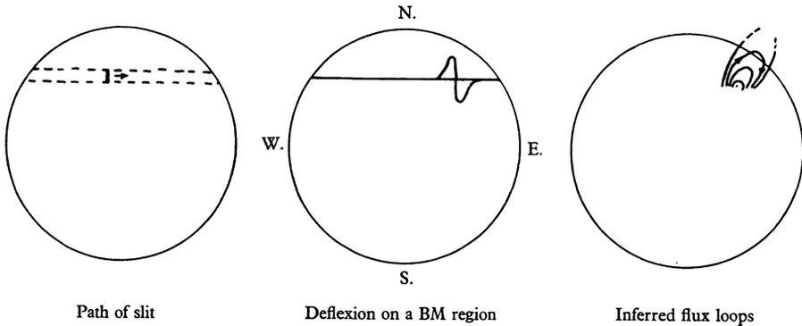
Fig. 1. Response trace of magnetograph as slit scans image.
