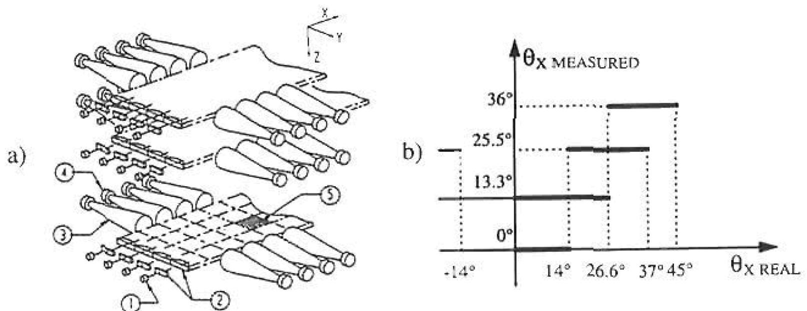
Figure 3. Recommended solution: a) implementation, with 1: laser diode, 2: collimating optics, 3: concentrator, 4: PIN photodiode and 5: basic measurement area, b) accuracy on the velocity direction projected on the x-axis
