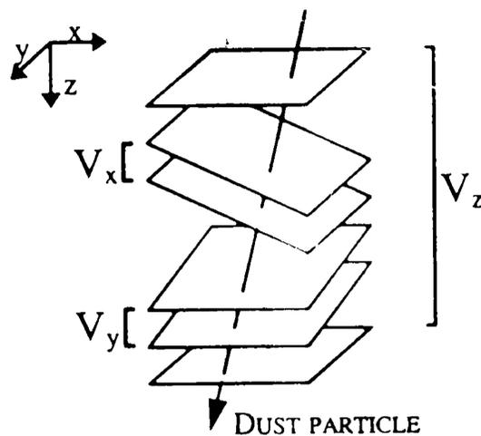
Figure 2. Geometry of inclined planes concept.
