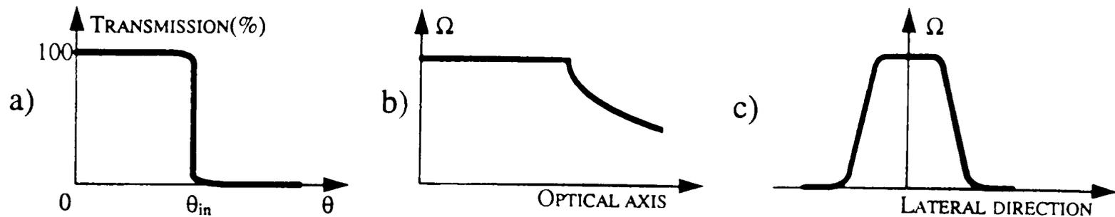
Figure 1. Properties of a concentrator: a) limited field-of-view, b) acceptance angle along the concentrator optical axis, c) acceptance angle orthogonally to the optical axis
