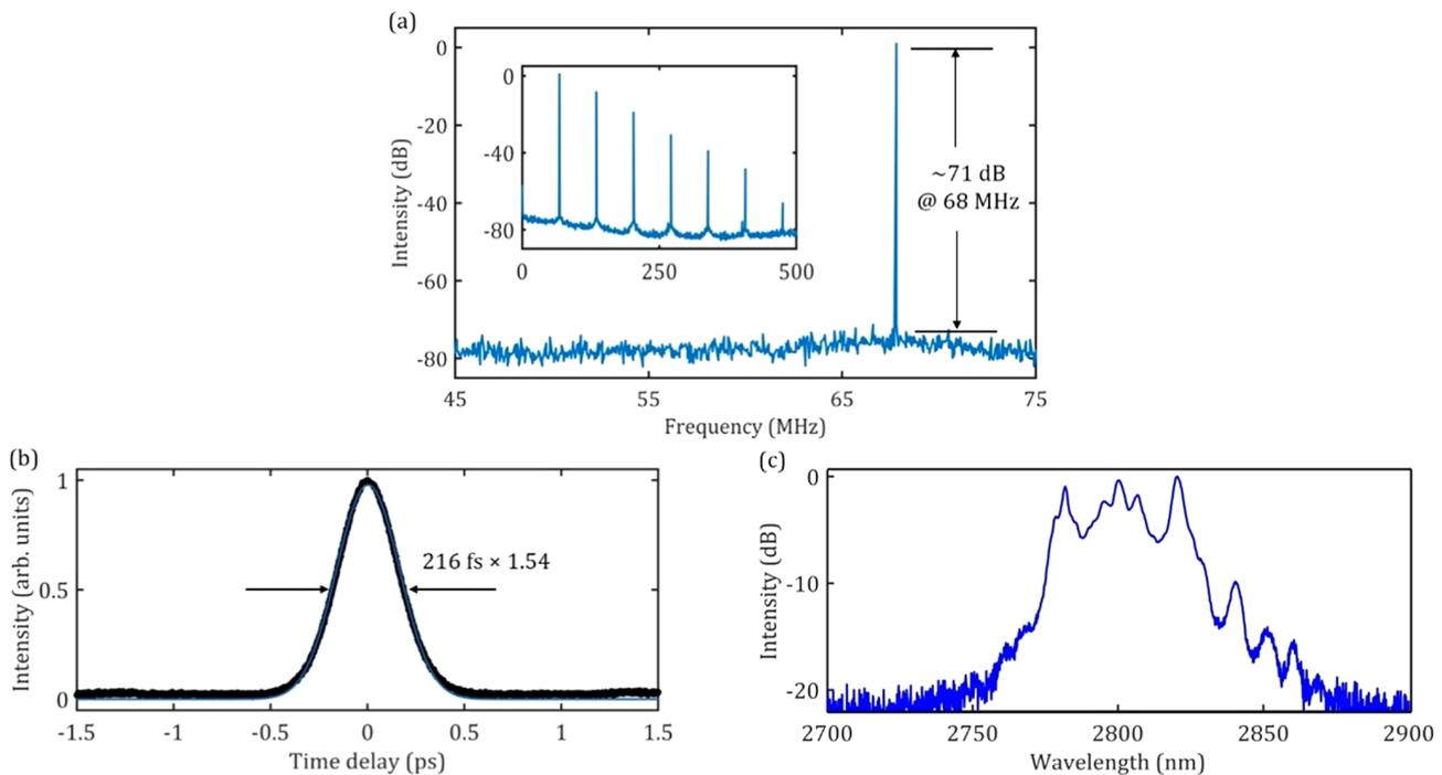
**Figure 4.** (a) Measured radio-frequency (RF) spectrum of the mode-locked pulses. Inset: RF spectrum with 500 MHz span. (b) Measured autocorrelation trace of the mode-locked pulses (black dots) with a  $\text{sech}^2$  fit (blue solid line). (c) Optical spectrum of mode-locked pulses. These results were measured under the average output power of 1.09 W.
