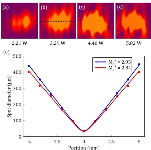
**Figure 2.** (a) The output beam pattern recorded in continuous-wave operation. (b)–(d) The output beam patterns recorded in spatiotemporal mode-locking operation at different pump powers. (e) The measured  $M^2$  factors of the output beam at pump power of 4.40 W in the spatiotemporal mode-locking operation.
