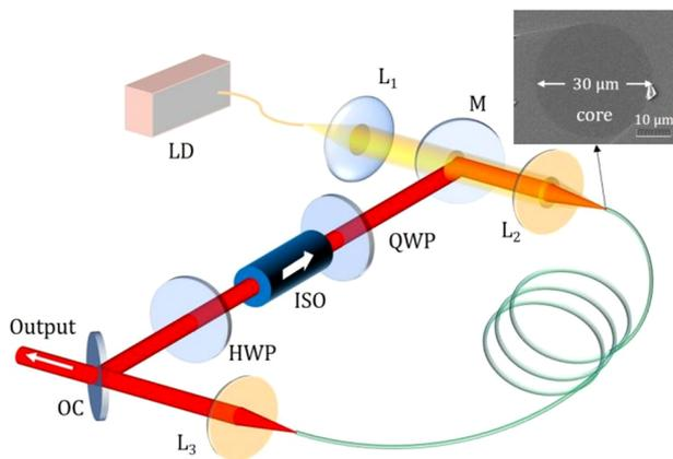
**Figure 1.** Schematic of the spatiotemporally mode-locked soliton Er:ZBLAN fiber laser. LD, laser diode;  $L_1$ , spherical lens;  $L_2$  and  $L_3$ , aspherical ZnSe lenses; M, dichroic mirror; OC, output coupler; HWP, half-wave plate; QWP, quarter-wave plate; ISO, isolator. Inset: the enlargement of the fiber facet obtained by a scanning electron microscope, showing a 30- $\mu\text{m}$  fiber core diameter.
