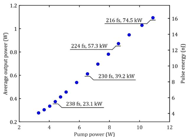
**Figure 5.** The output average power and pulse energy versus pump power for the spatiotemporally mode-locked soliton fiber laser. The recorded data are the corresponding pulse duration and peak power.
