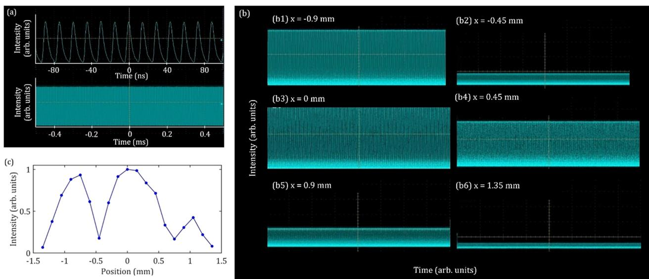
**Figure 3.** (a) Recorded mode-locked pulse trains in the 200 ns and 1 ms time scales. (b) Sampled pulse trains at different spatial positions. (c) Intensities of sampled pulse trains versus spatial positions.
