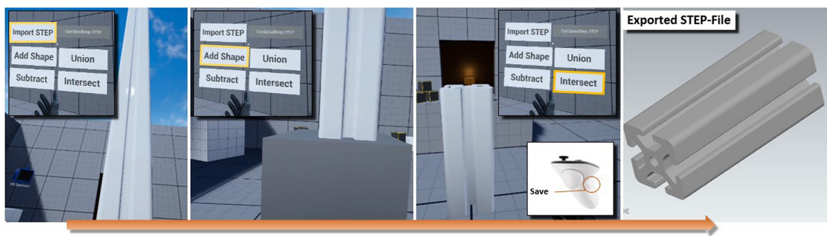
Figure 5. Example manipulation of an imported STEP-file with subsequent STEP-file export
