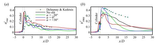
Figure 11. Maximum r.m.s. velocity fluctuations along the line of constant x/D for different slit-offset angles: (a) axial velocity fluctuations ( $u'_{rms}$ ) and (b) transverse velocity fluctuations ( $v'_{rms}$ ). (The trend is duly compared with the results obtained by Delaunay & Kaiktsis (2001) for the stationary cylinder at Re = 90).
