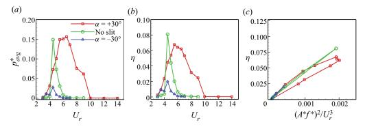
Figure 15. Effect of slit-offset angle on the harnessed power: (a) non-dimensional average extracted power, (b) power extraction efficiency and (c) variation of power extraction efficiency against the combined VIV parameter ( $m^* = 10, \zeta = 0.02, Re = 500$ ).
