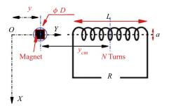
Figure 2. Cylinder-magnet arrangement layout for energy harvesting via electromagnetism.
