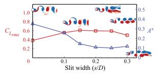
Figure 5. Effect of slit width on the lift force and corresponding transverse oscillations of the slit cylinder with the visualization of the vortex shedding via means of the instantaneous spanwise vorticity ( $-5 \le \omega_z \le +5$ );  $m^* = 10$ ,  $U_r = 5$ ,  $\zeta = 0.02$ ,  $\alpha = 0^\circ$  and Re = 500.
