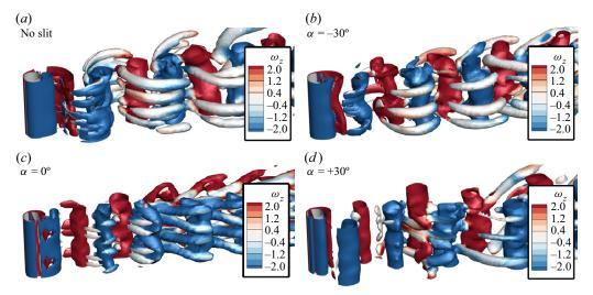
Figure 7. Three-dimensional structures behind the transversely oscillating circular slit cylinder for various slit-offset angles via means of the isosurfaces of eigenvalue  $e_2 = 0.02$  ( $m^* = 10$ ,  $U_r = 5$ ,  $\zeta = 0.02$  and Re = 500).
