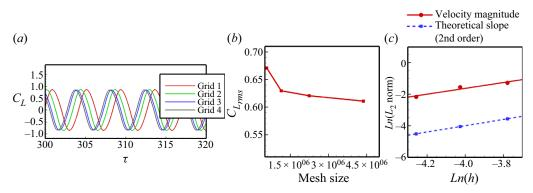
Figure 3. Grid independence study at Re = 500 for an unconfined cylinder with a normal slit: (*a*) temporal variation of the lift coefficient ( $C_L$ ), (*b*)  $C_{L_{rms}}$  variation with the mesh size, (*c*)  $L_2$  norm against the grid spacing *h* compared with the theoretical slope for second order [ $m^* = 10$ ,  $U_r = 5$ ,  $\zeta = 0.02$ ,  $\alpha = 0^\circ$  and Re = 500].
