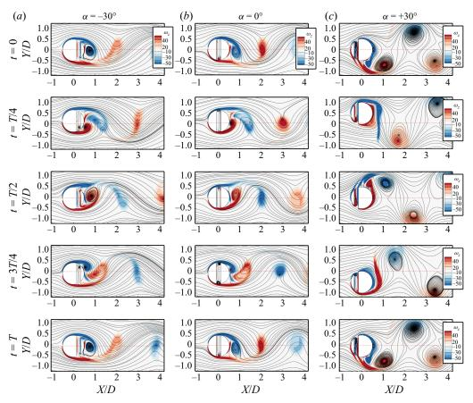
Figure 9. Temporal evolution of the instantaneous velocity streamlines for one complete oscillation cycle at different slit-offset angles: (a)  $\alpha = -30^{\circ}$ , (b)  $\alpha = 0^{\circ}$  and (c)  $\alpha = +30^{\circ}$ ;  $m^* = 10$ ,  $U_r = 5$ ,  $\zeta = 0.02$ , s/D = 0.20 and Re = 500.
