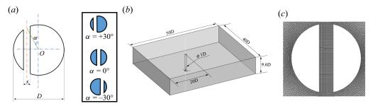
Figure 1. (*a*) The definition of the slit-offset angle, (*b*) schematic of the computational domain for the study, (*c*) zoomed view of the computational mesh near the slit cylinder.
