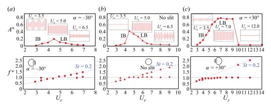
Figure 13. Effect of reduced velocity on oscillation amplitude and frequency response for different slit-offset angles: (a)  $\alpha = -30^{\circ}$ , (b) no-slit case and (c)  $\alpha = +30^{\circ}$ ;  $m^* = 10$ ,  $\zeta = 0.02$ , Re = 500.
