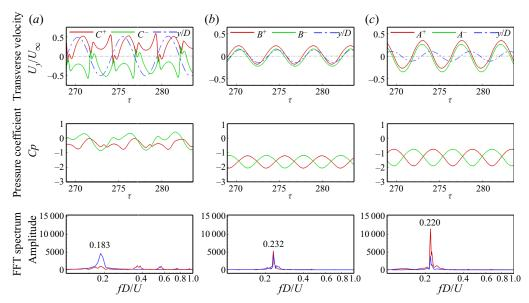
Figure 10. Development of suction and blowing phenomena inside the slit via the temporal evolution of pressure and velocity at the slit openings (top slit opening: red solid line, bottom slit opening: green solid line, the blue dashed dotted line shows the corresponding oscillation amplitude) for different slit-offset angles: (a)  $\alpha = +30^{\circ}$ , (b)  $\alpha = 0^{\circ}$  and (c)  $\alpha = -30^{\circ}$ ;  $m^* = 10$ ,  $U_r = 5$ ,  $\zeta = 0.02$ , s/D = 0.20 and Re = 500.
