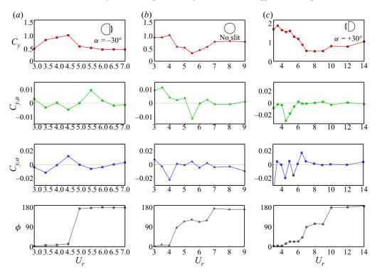
Figure 14. Variation of the lift coefficient ( $C_y$ ) and its corresponding component in phase with velocity ( $C_{y,u}$ ) and displacement ( $C_{y,a}$ ), and the phase difference between the lift and the y displacement for different slit-offset cases: (a)  $\alpha = -30^{\circ}$ , (b) no-slit case and (c)  $\alpha = +30^{\circ}$ ;  $m^* = 10$ ,  $\zeta = 0.02$ , Re = 500.
