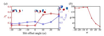
Figure 8. Effect of the slit-offset angle: (*a*) variation of transverse oscillation amplitude and the r.m.s. of the lift coefficient for different slit-offset angles (with visualization of the instantaneous vorticity  $(-10 \le \omega_z \le +10)$ ), (*b*) variation of the phase difference between the lift force and the oscillation amplitude ( $\phi$ );  $m^* = 10$ ,  $U_r = 5$ ,  $\zeta = 0.02$  and Re = 500.
