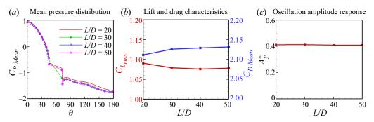
Figure 16. Domain independence study for the 1-DOF VIV slit cylinder: mean pressure distribution over the cylinder surface, the lift and drag characteristics for different domain length, and the VIV oscillation amplitude response;  $m^* = 10$ ,  $U_r = 5$ ,  $\zeta = 0.02$ , Re = 500, s/D = 0.2,  $\alpha = +30^\circ$ .
