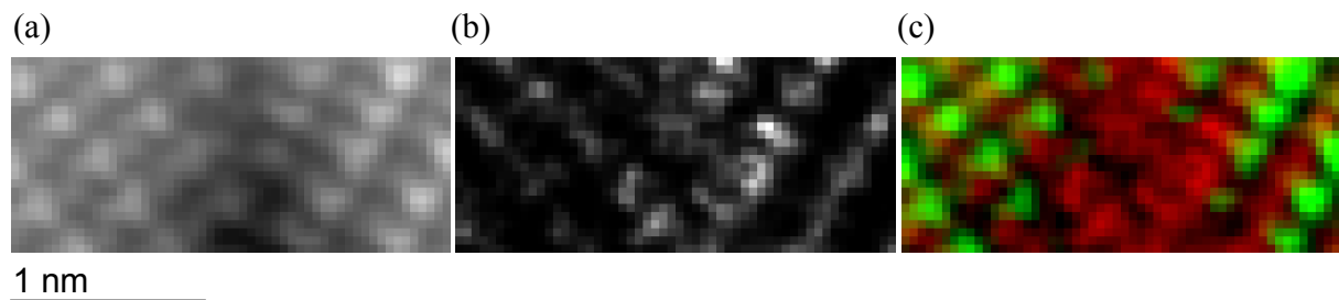
Figure 2: (a) HAADF STEM image of the \text{SrTiO}_3 \Sigma 3(112)[-110] grain boundary acquired simultaneously with EELS data. (b) Ti spectrum image corresponding to the same area as the HAADF image. (c) Ti spectrum image (red) overlaid onto the HAADF STEM image (green) (colour on CD proceedings). Note that a non-linear contrast scale has been employed when displaying the images. The area shown is similar to that indicated by the dashed rectangle in figure 1a.
