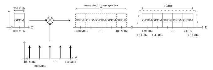
Fig. 3. Frequency plan for the multiplication of the OFDM signal with the frequency comb.
