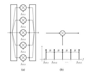
Fig. 2. Methods to multiply with a frequency comb. (a) Multiplication using multiple mixers and multiple single frequency sources. (b) Direct multiplication with the frequency comb in a single multiplier.
