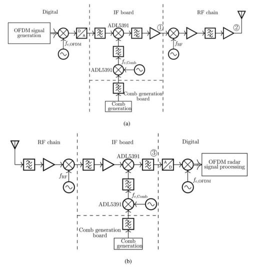
**Fig. 6.** Radar architecture (based on [1]): (a) transmitter, (b) receiver.
