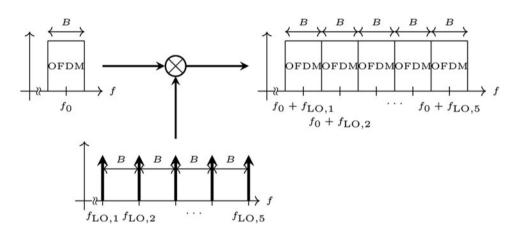
Fig. 1. Multiplication of the OFDM signal with the frequency comb (based on [1]).
